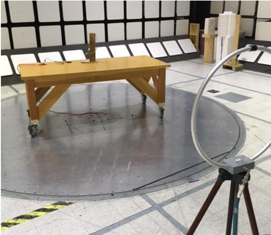
Figure 9 – Radiated Emissions Testing, 9 kHz – 30 MHz
