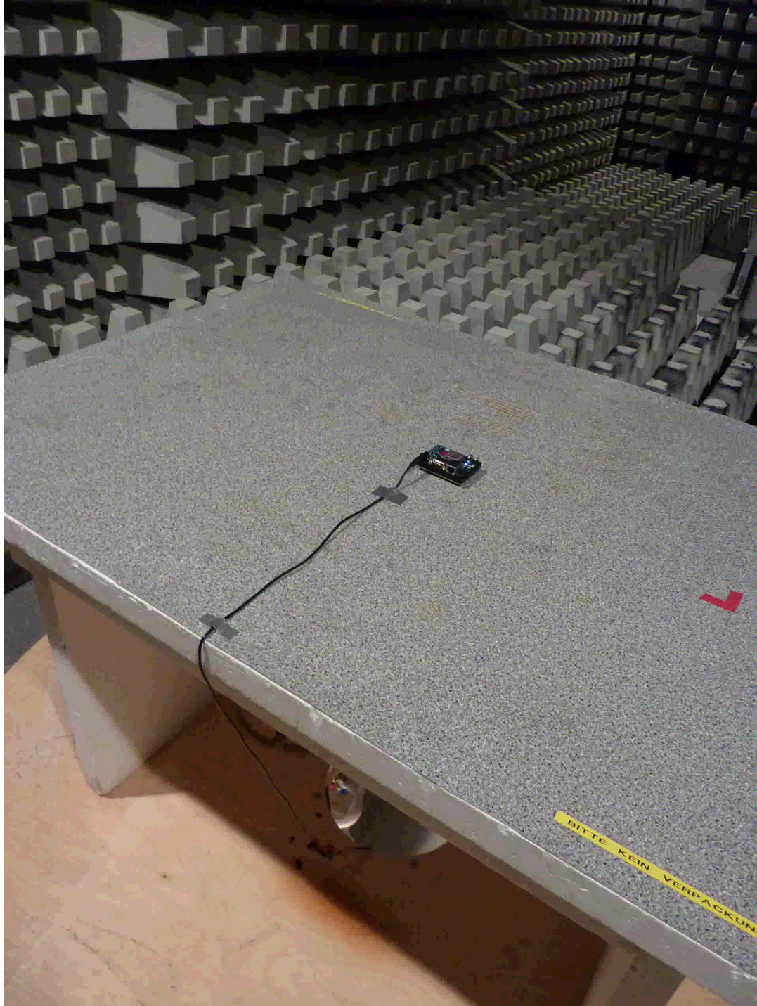
101336_7.jpg cB-OBC001i, test set-up fully anechoic chamber
