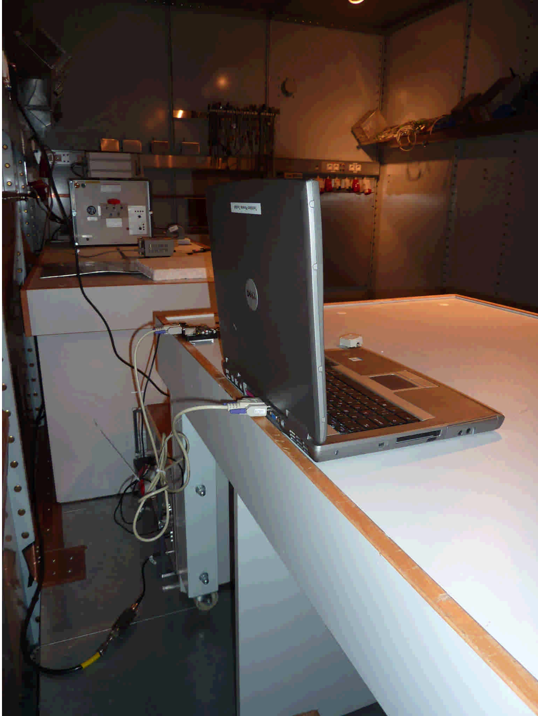
101336_14.jpg cB-OBC001i, test set-up shielded chamber
