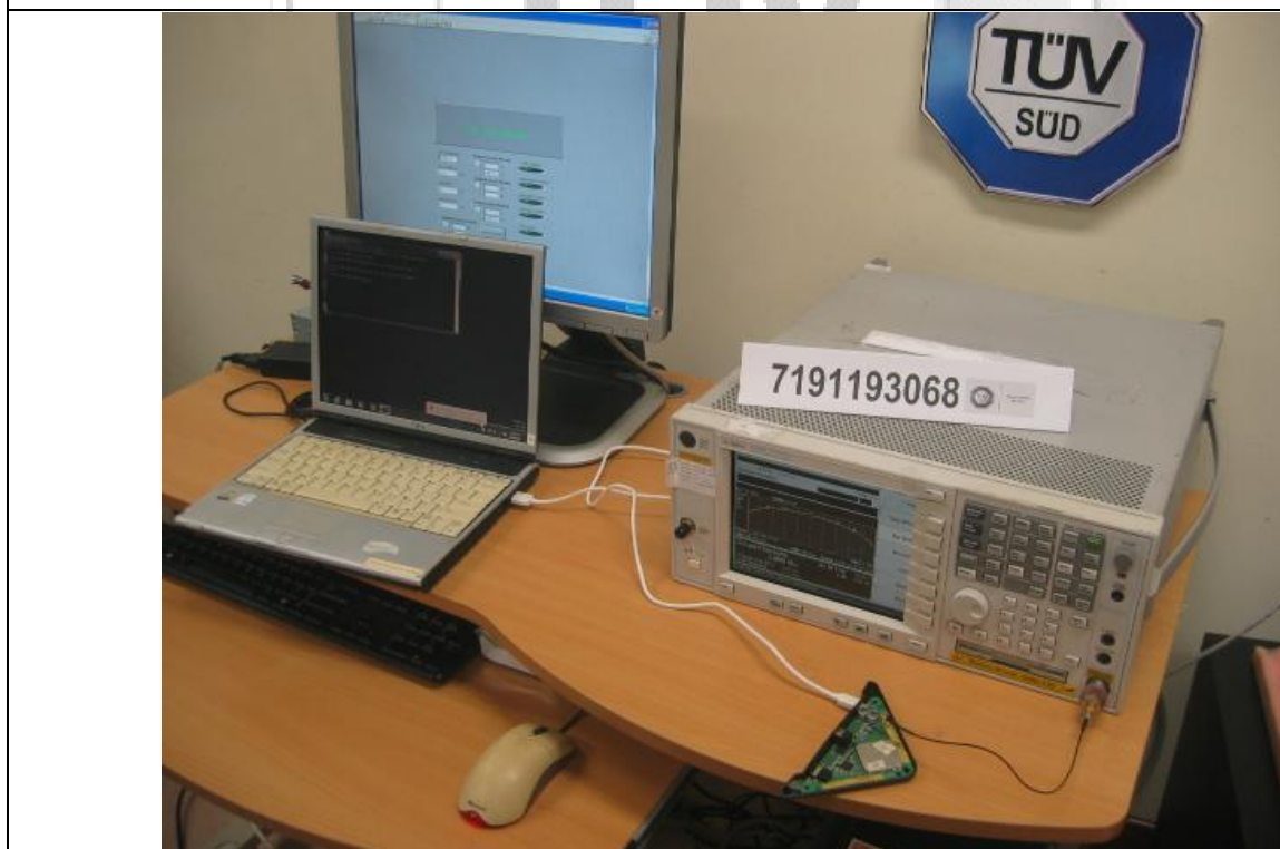
Average Frequency Dwell Time Test Setup
