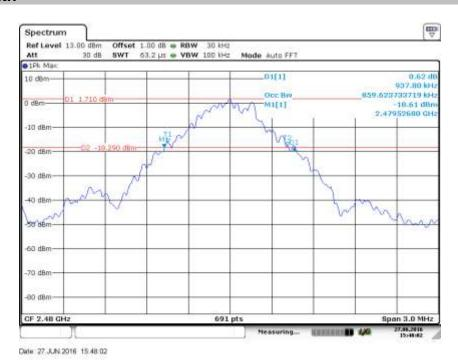
Bluetooth Mode  $\pi/4$ -DQPSK Modulation test result
