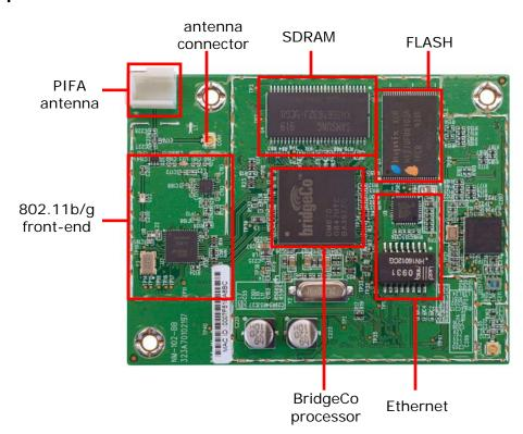
**Note:** Components and Socket to the right of the Ethernet and Flash sections are not installed in production modules. Please see Section 3.3 for example production module top view picture.
