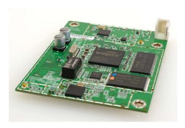
Complete audio networking system on a small module
