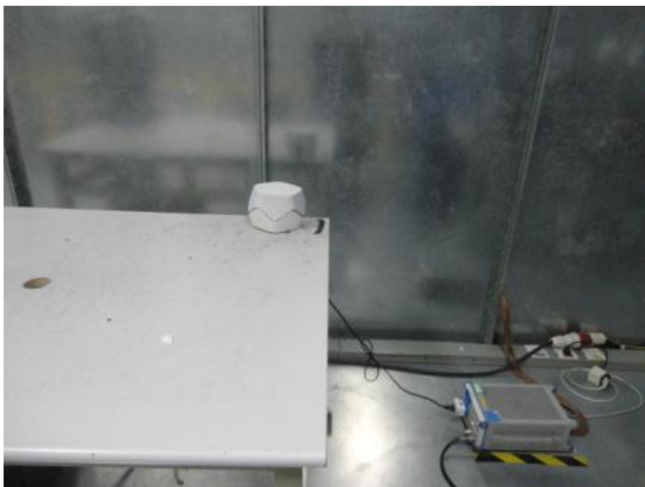
Photograph 4: Set-up for Conducted Emissions
