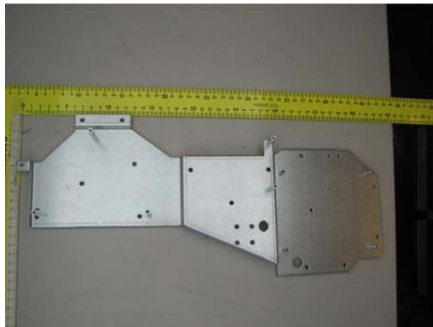
PSU / Main board mounting frame top
