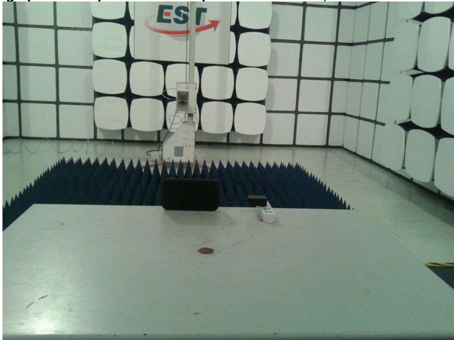
Photograph 3: Set-up for Radiated Spurious Emissions, Above 1GHz
