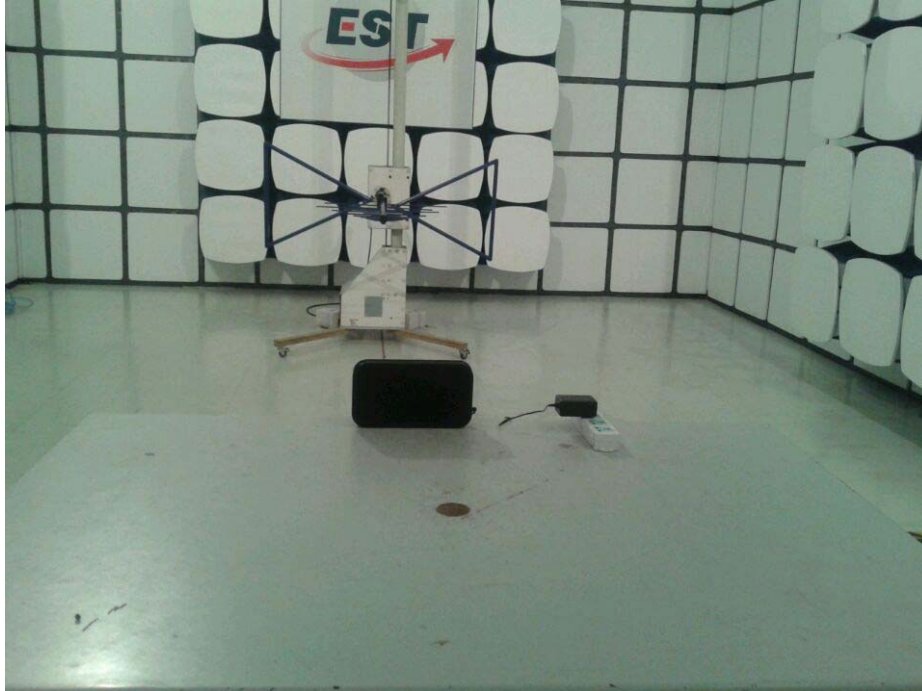
Photograph 2: Set-up for Radiated Spurious Emissions, 30MHz-1GHz
