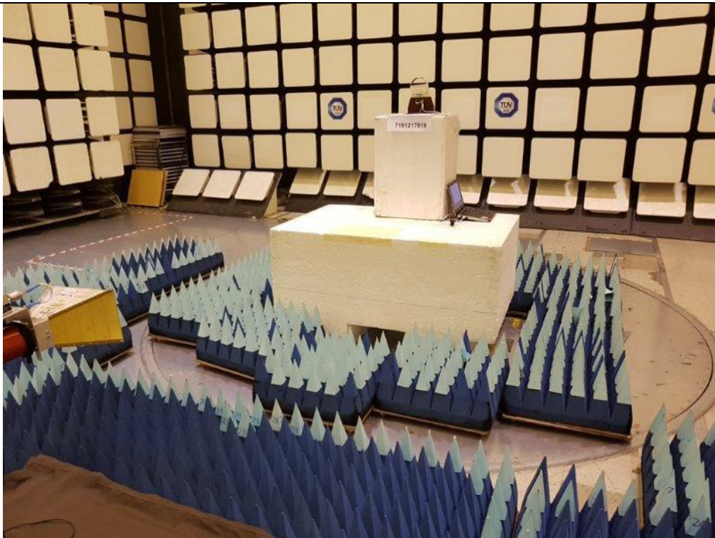
Band Edge Compliance (Radiated) Test Setup
