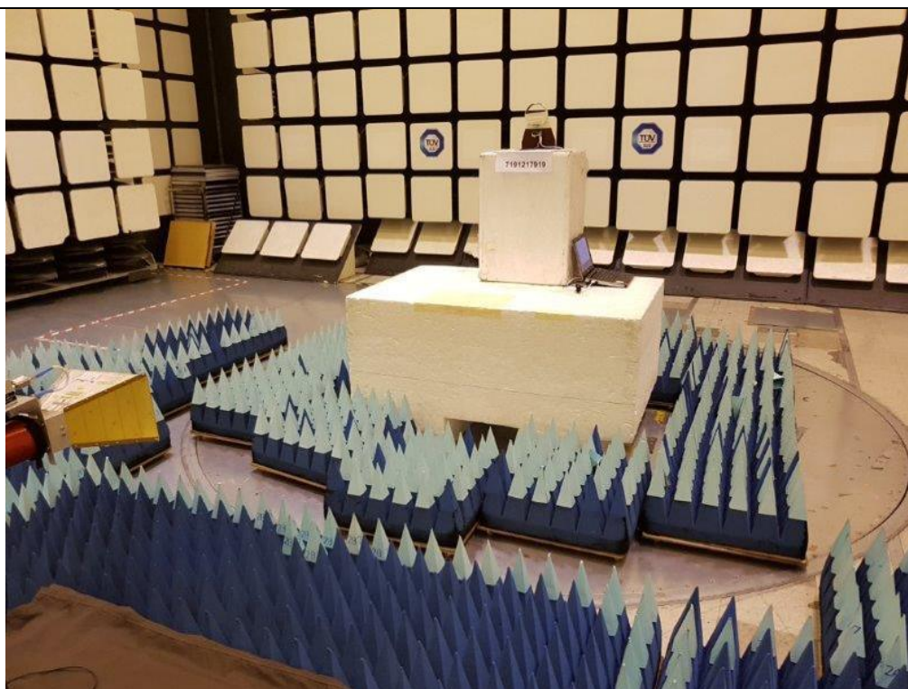
Band Edge Compliance (Radiated) Test Setup
