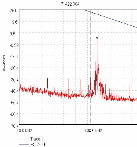
Start 9.0 kHz; Stop 490.0 kHz - Log Scale
