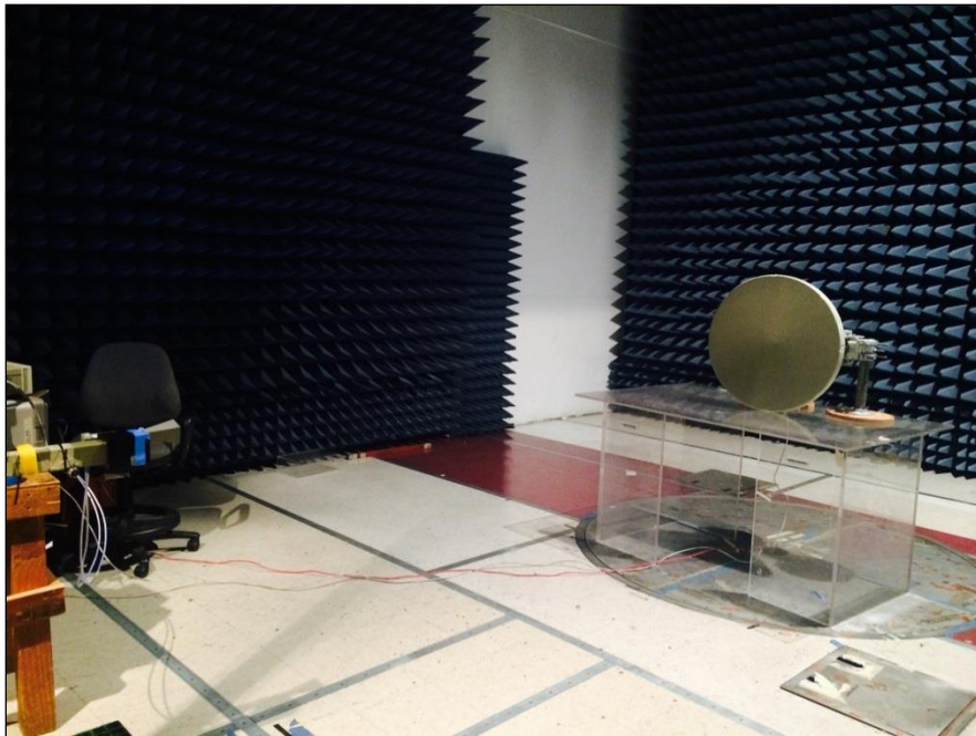
Photograph 6. Radiated Spurious Emissions, Test Setup, Above 18-40GHz
