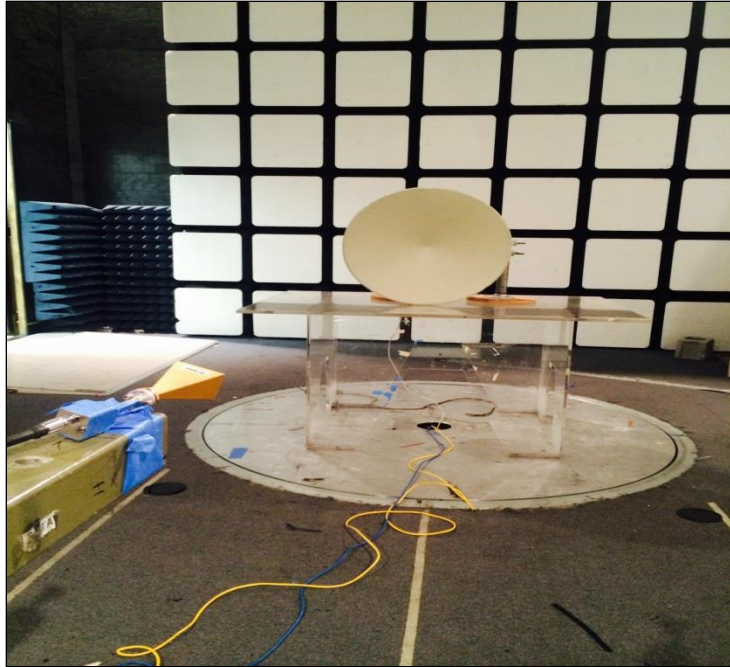
Photograph 7. Radiated Spurious Emissions, Test Setup, Above 40 GHz
