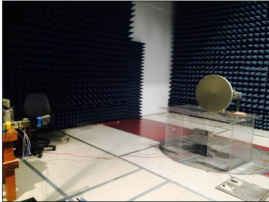
Photograph 6. Radiated Spurious Emissions, Test Setup, Above 18-40GHz
