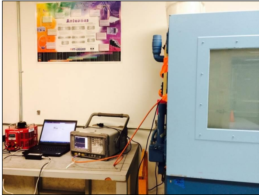
Photograph 2. Frequency Tolerance, Test Setup
