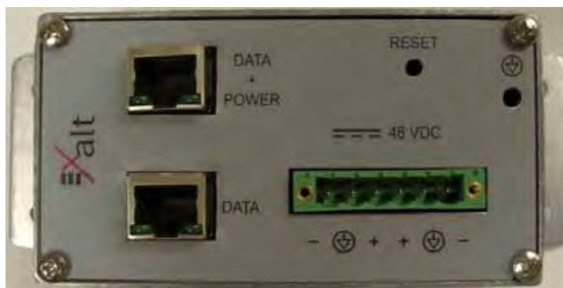
Figure 15 Power injector connectors
