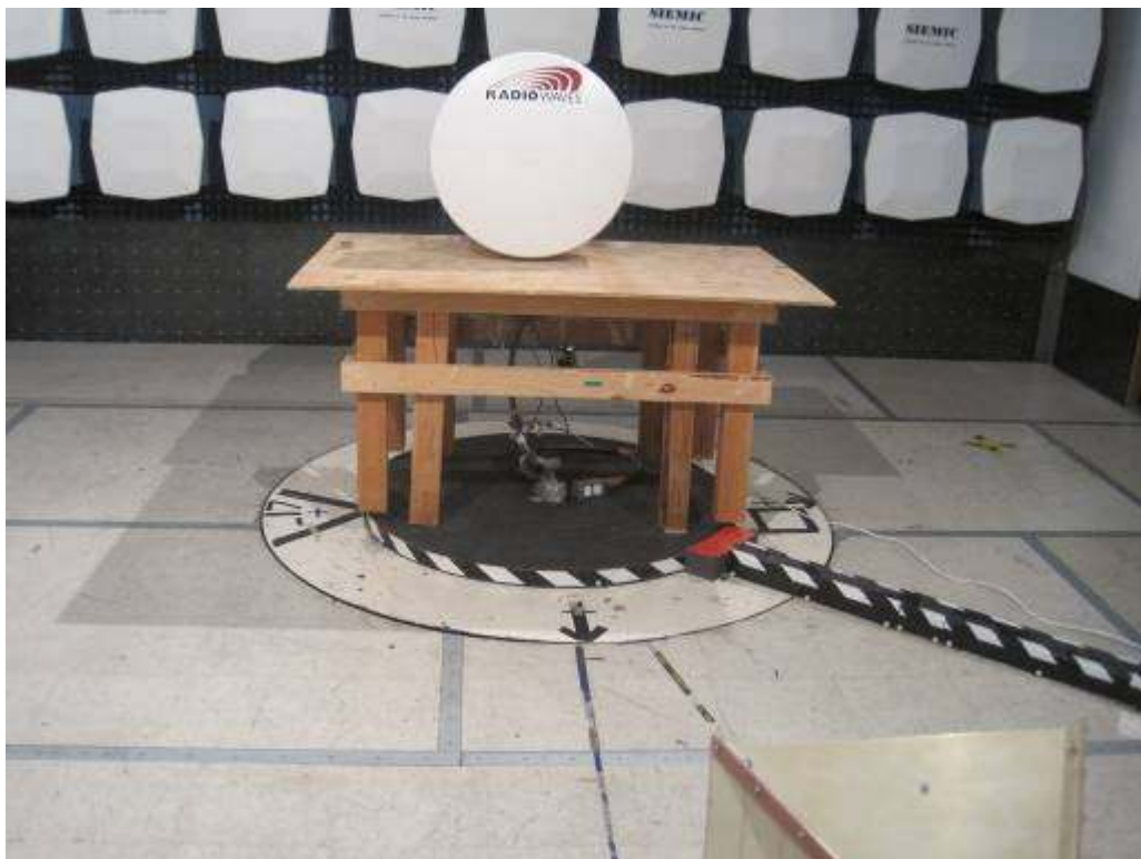
Radiated Emission (Above 1GHz) – Rear View Tested with Antenna model: HP2-26EX with gain 41.1dBi
