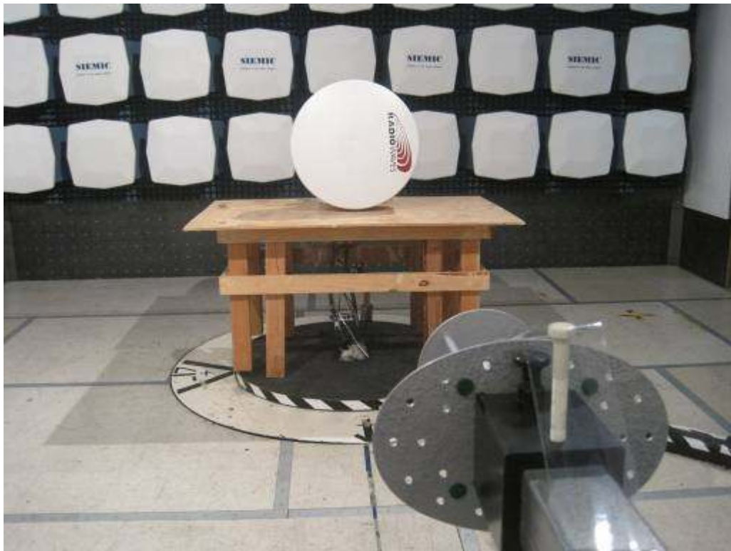
Radiated Emission (Above 18GHz) – Front View Tested with Antenna model: HP2-26EX with gain 41.1dBi
