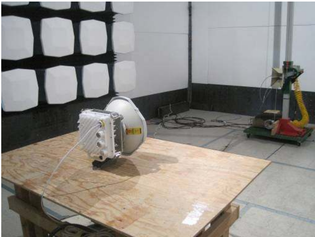
Radiated Emission (Above 1GHz) – Rear View Tested with Antenna Model: HPCPE-276EX with gain 35.9dBi
