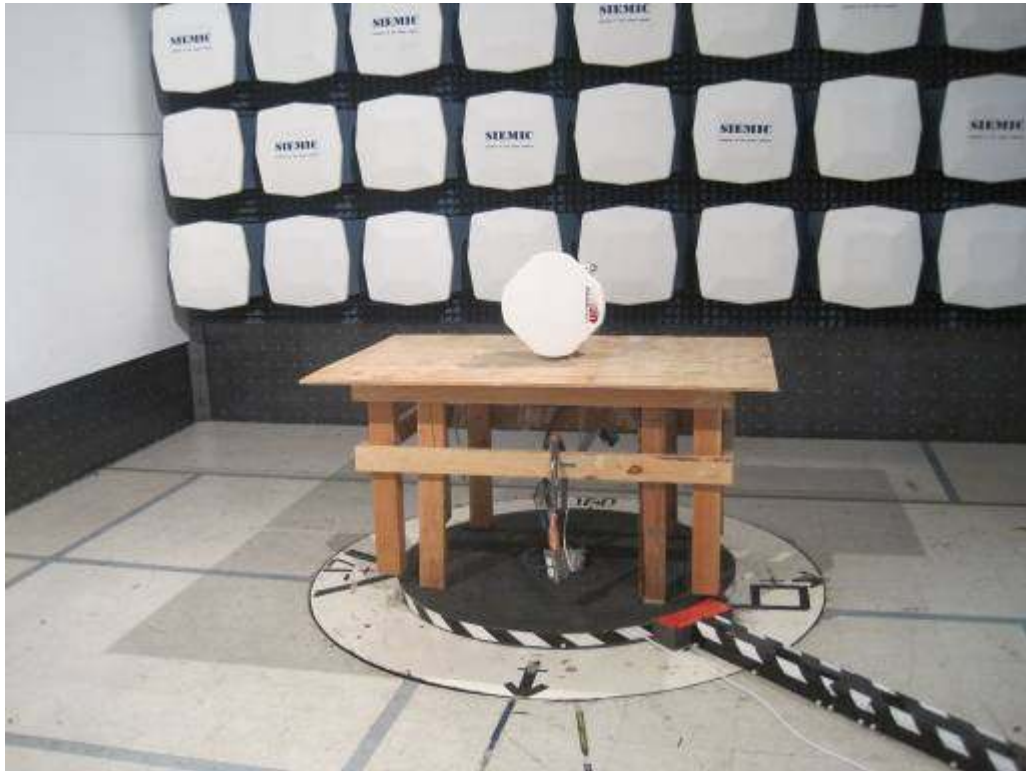
Radiated Emission (Above 18GHz) – Front View Tested with Antenna Model: HPCPE-276EX with gain 35.9dBi
