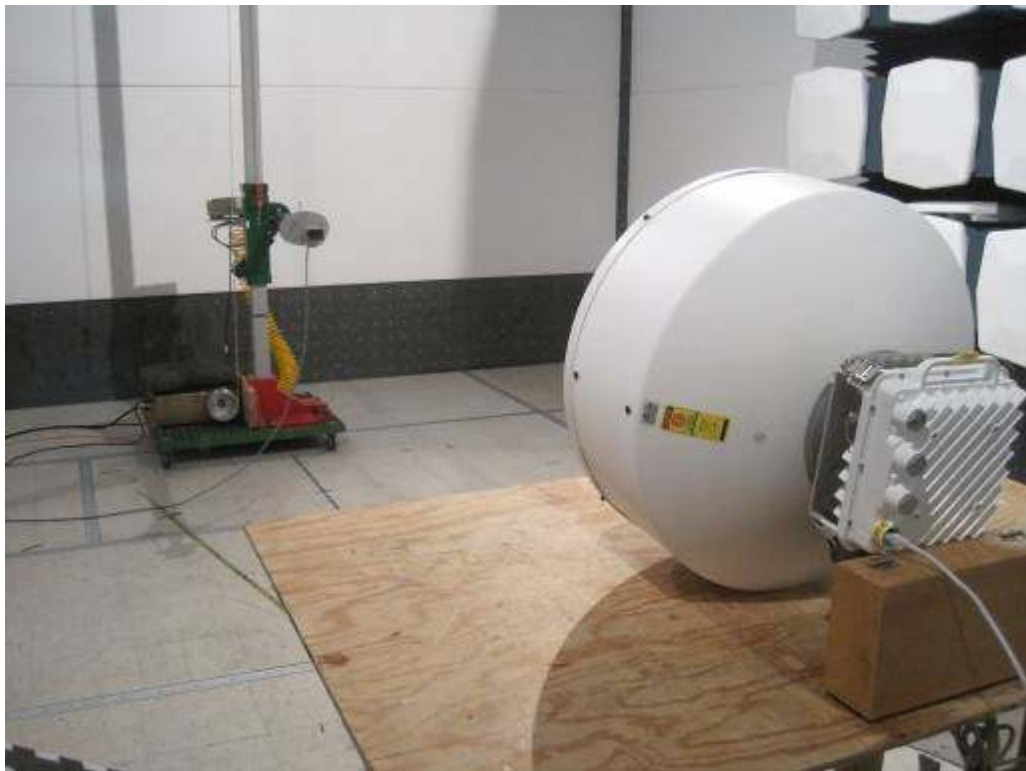
Radiated Emission (Above 18GHz) – Rear View Tested with Antenna model: HP2-26EX with gain 41.1dBi
