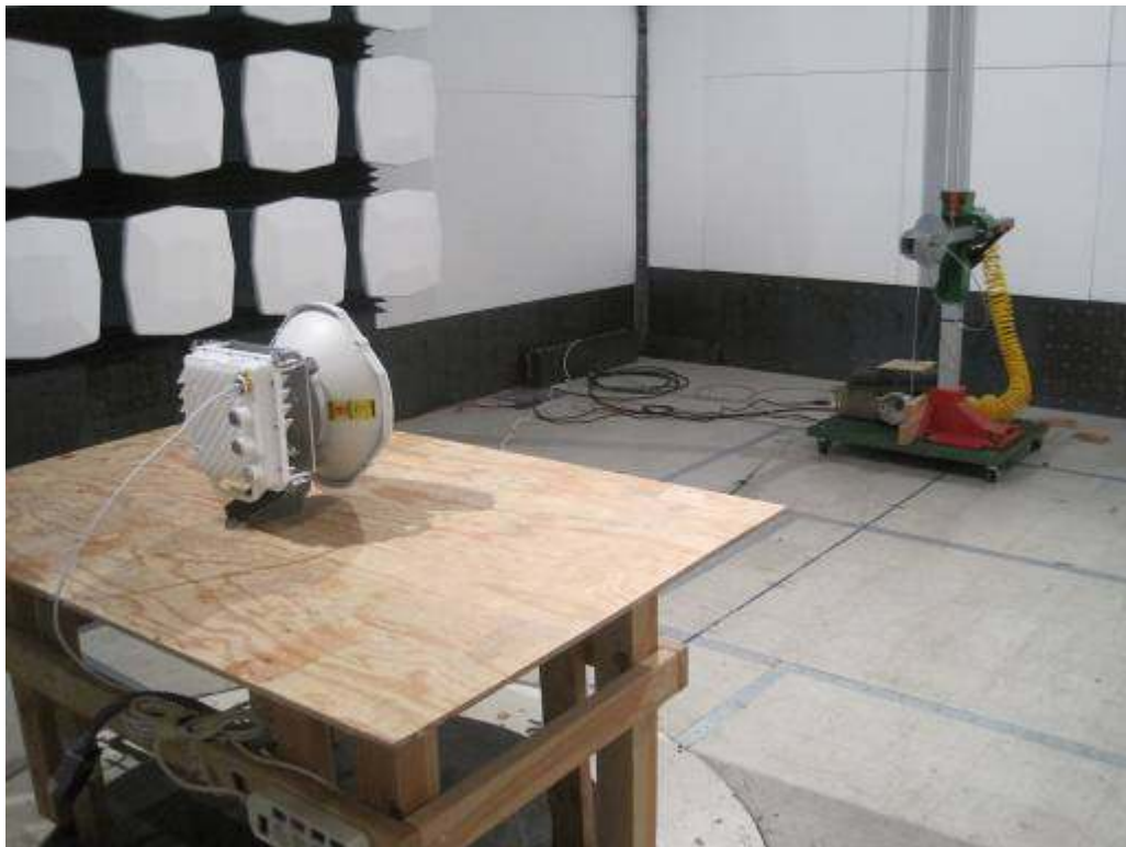
Radiated Emission (Above 18GHz) – Rear View Tested with Antenna Model: HPCPE-276EX with gain 35.9dBi
