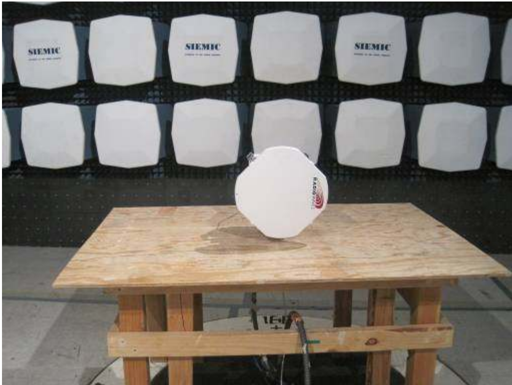
Radiated Emission (Above 1GHz) – Front View Tested with Antenna Model: HPCPE-276EX with gain 35.9dBi
