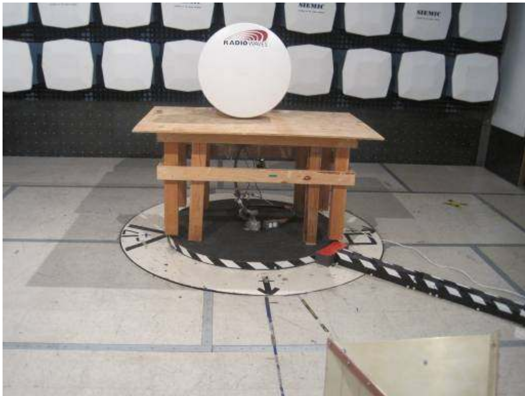
Radiated Emission (Above 1GHz) – Front View Tested with Antenna model: HP2-26EX with gain 41.1dBi
