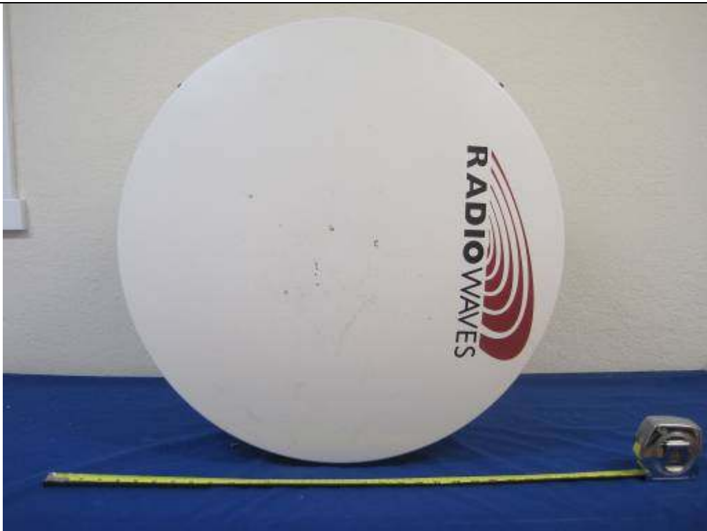
Antenna model: HP2-26EX with gain 41.1dBi
