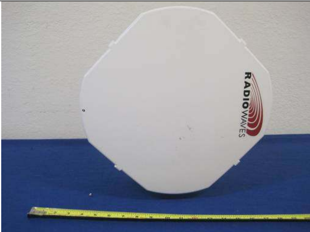
Antenna Model: HPCPE-276EX with gain 35.9dBi
