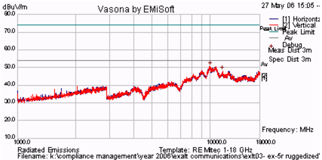
5,296 MHz Radiated Emissions for 28 dBi Antenna 15 MHz Bandwidth QPSK
