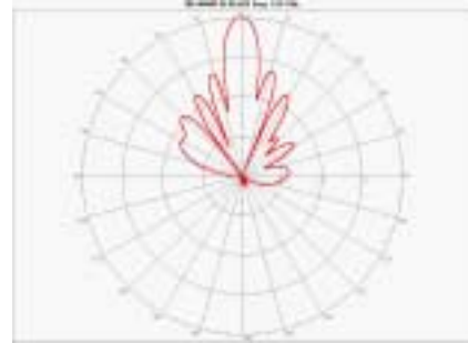
Elevation Radiation Pattern Midband Freq. 5.35 GHz
