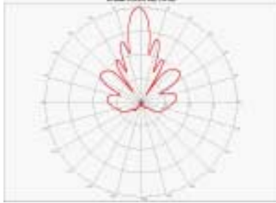
Azimuth Radiation Pattern Midband Freq. 5.35 GHz
