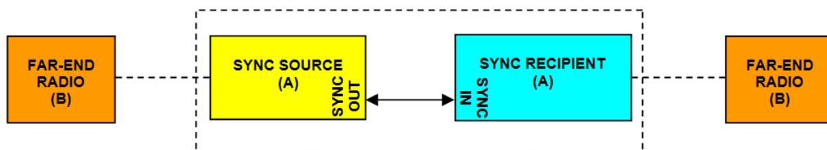
Figure 4 Basic radio interconnectivity using internal synchronization
