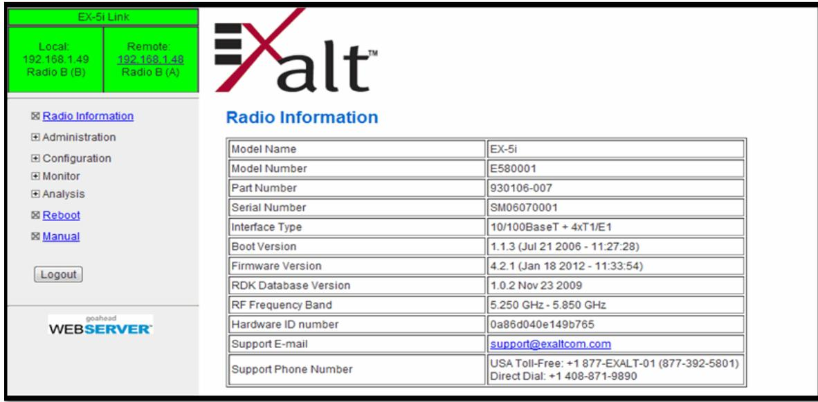
The screenshot shows the Exalt web interface. At the top, there is a green header with 'EX-5i Link' and two columns for 'Local' and 'Remote' radio information. Below this is a navigation menu with options like 'Radio Information', 'Administration', 'Configuration', 'Monitor', 'Analysis', 'Reboot', and 'Manual'. The main content area is titled 'Radio Information' and contains a table with the following data:
