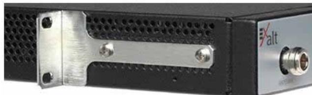
*Figure 11 Front projection mount configuration*
