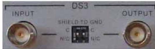
Figure 17 EX-5i-DS3 connectors and grounding switches
