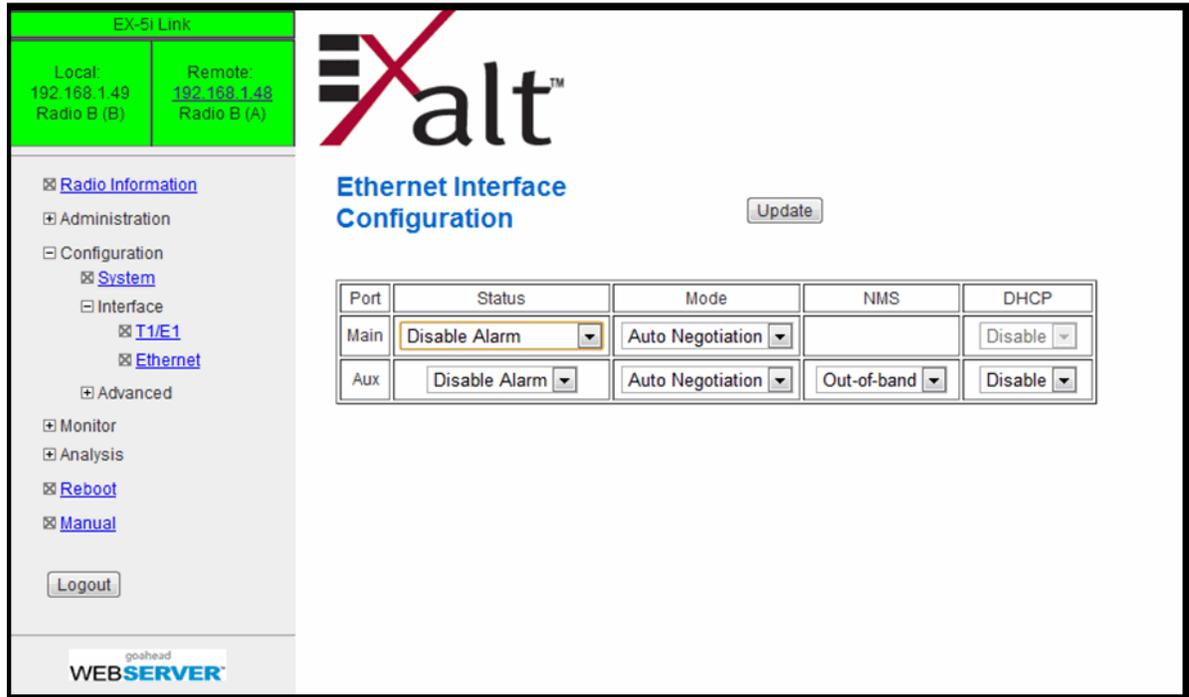
Figure 36 Ethernet Interface Configuration page
