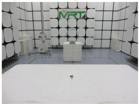
Description: Radiated Emission Test Setup for Below 30MHz-1GHz
