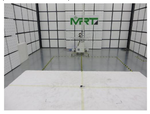
Description: Radiated Emission Test Setup for 1GHz ~ 6GHz
