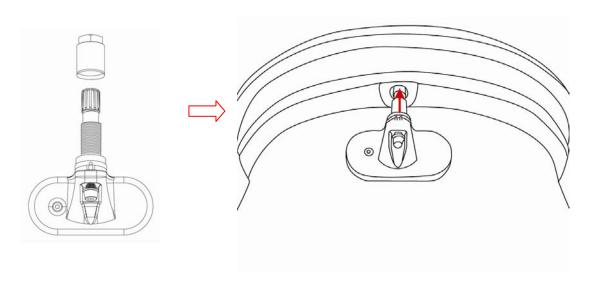
② Screw the sensor nut by hand, and employ 12mm sleeve to tighten it (torque force 4N.M).
