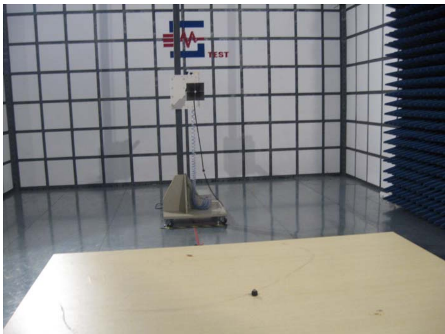
Radiation Emission Test Setup (Above 1GHz)
