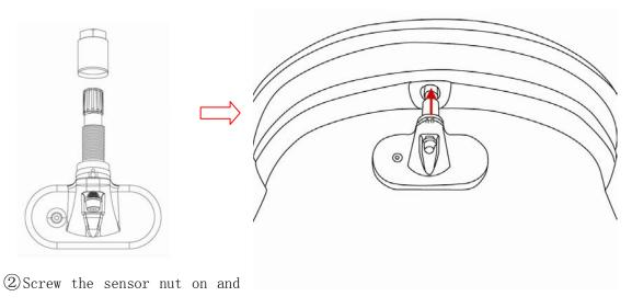
tighten it with 12mm sleeve. Torque is 4N.m( $\pm 0.5$ ) ;
