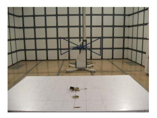
Radiation Emission Test Setup (Above 1GHz)
