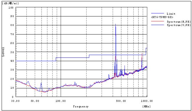
Plot of Radiation Emissions Test
