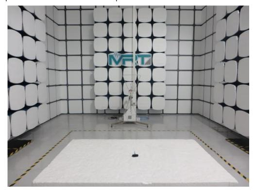
Description: Radiated Emission Test Setup for  $1\text{GHz} \sim 18\text{GHz}$
