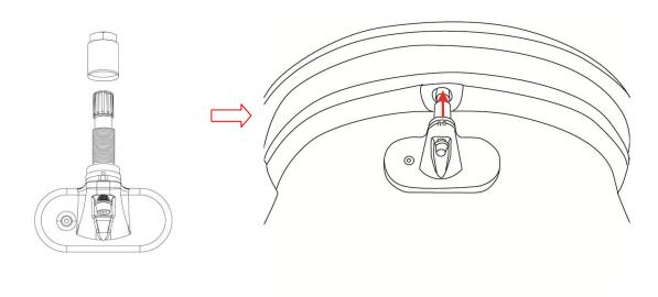
② Screw the sensor nut by hand, and employ 12mm sleeve to tighten it (torque force 4N.M).
