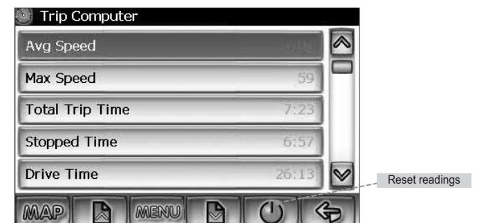
Scroll the Up or Down arrow button to choose the field then press to reset current reading.
