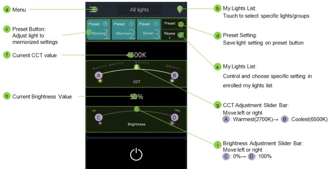
**Light Control:** Adjust Correlated Color Temperature (CCT) and Brightness through simple touch controls.
