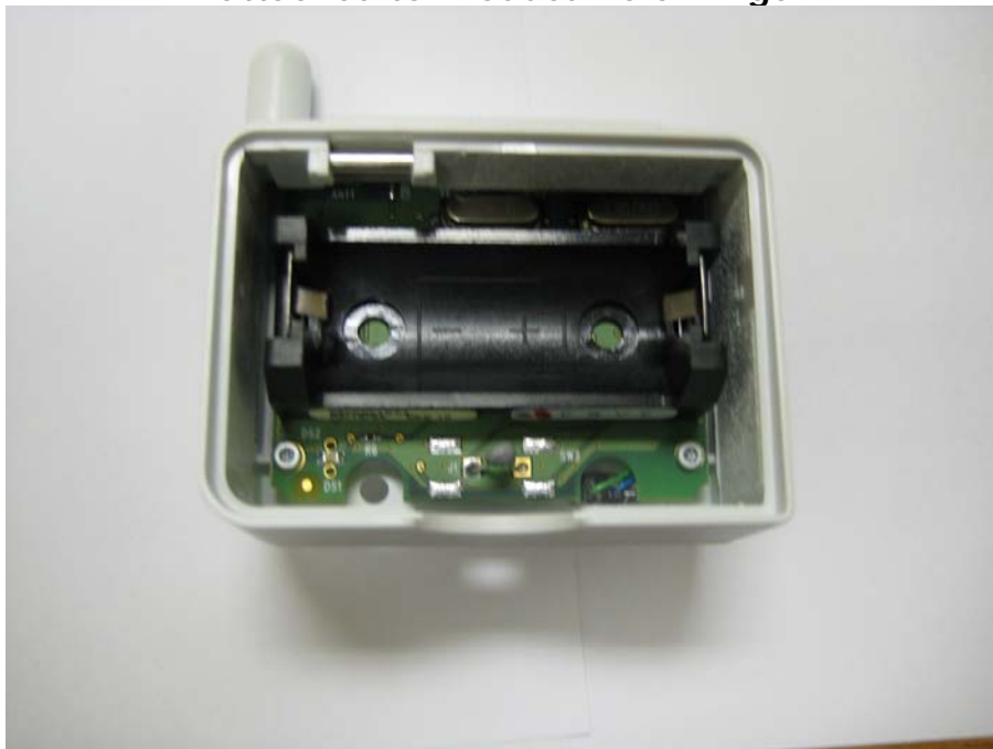
Open for Inspection – Battery Compartment
