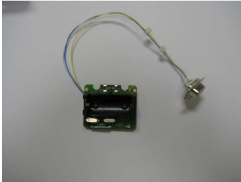
Open for Inspection #1, Showing Connection/Wire Attached
