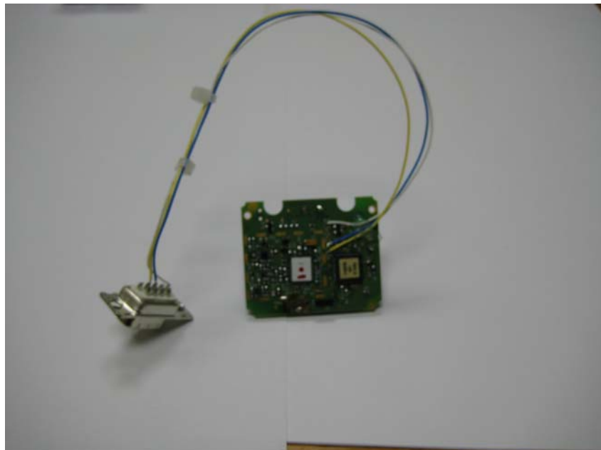
Open for Inspection #2, RF Section -Showing Connection/Wire Attached
