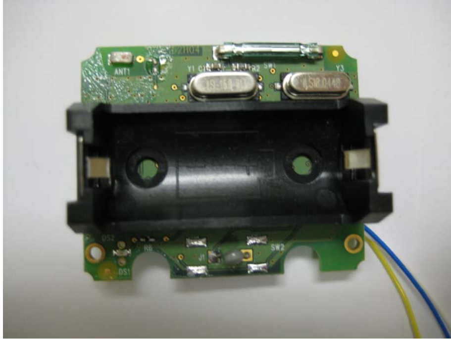
Close Up of Battery Compartment
