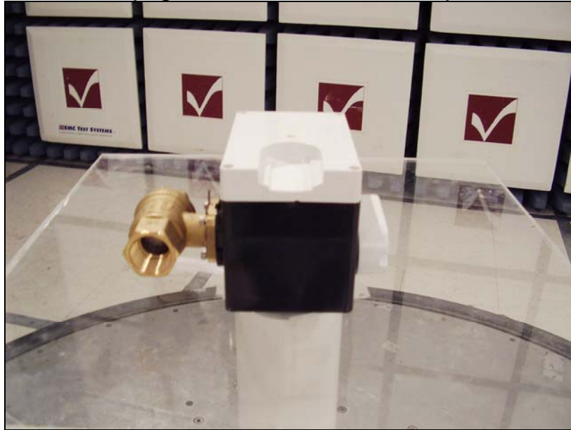
View of the EUT setup in Horizontal orientation (Highest emissions measured)
