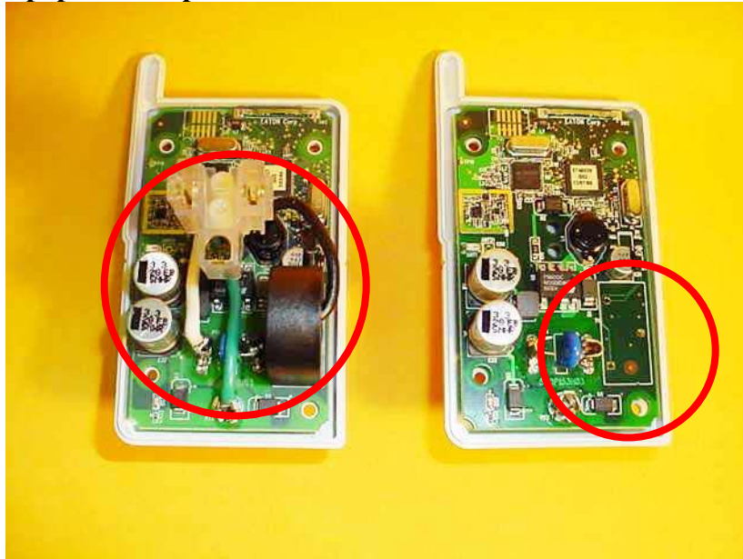
The Eaton “Appliance Monitor” (on the left) and the “Range Extender” (on the right) Different population options are identified within the circles for each device.
