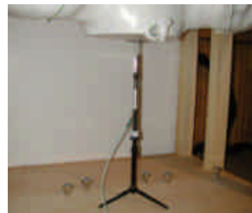
Figure 12.1 Dipole Validation Test Setup
