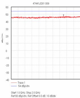
RBW 1.0 MHz; VBW 1.0 MHz; Att 0 dB; Swp 20.0 mS Peak 1.756 GHz, 47.56 dBµV/m Display Line: 54 dBµV/m; Transducer Factors: 1 to 2 22/09/2005 16:14:51
