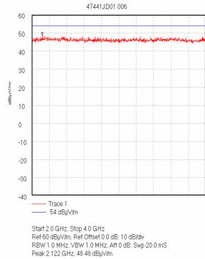
Display Line: 54 dBµV/m; Transducer Factors: 2 to 4 22/09/2005 15:59:49
