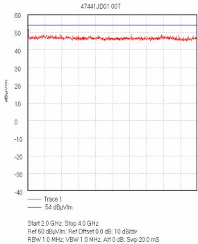
Start 2.0 GHz; Stop 4.0 GHz Ref 60 dBµV/m; Ref Offset 0.0 dB; 10 dB/div RBW 1.0 MHz; VBW 1.0 MHz; Att 0 dB; Swp 20.0 mS Peak 2.007 GHz, 49.57 dBµV/m Display Line; 54 dBµV/m; Transducer Factors: 2 to 4 22/09/2005 16:05:28
