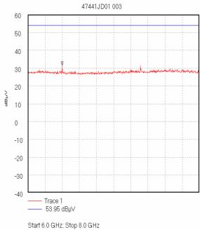
Ref 60 dBµV; Ref Offset 0.0 dB; 10 dB/div RBW 1.0 MHz; VBW 1.0 MHz; Att 10 dB; Swp 50.0 mS Peak 6.4 GHz, 31.67 dBµV Display Line: 53.95 dBµV; Transducer Factors: 6G-8G\_Horn(@0,7m,3m\_cable,A1534) 21/10/2005 10:46:47
