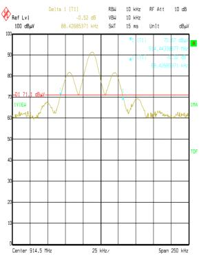
47441JD01 Radiometrix EUT: RPM3-914-17-ANT FCC Part 15.249 Comment A: 20dB Bandwidth EUT transmitting at Max Frequency Squarенave Modulated Carrier
