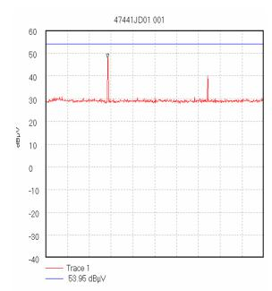
Start 4.0 GHz; Stop 6.0 GHz Ref 60 dBµV; Ref Offset 0.0 dB; 10 dB/div RBW 1.0 MHz; VBW 1.0 MHz; Att 10 dB; Swp 50.0 mS Peak 4.57 GHz, 47.67 dBµV Display Line: 53.95 dBµV; Transducer Factors: 4G-6G\_Horn(@1m,3m\_cable,A1534) 21/10/2005 10:06:32
