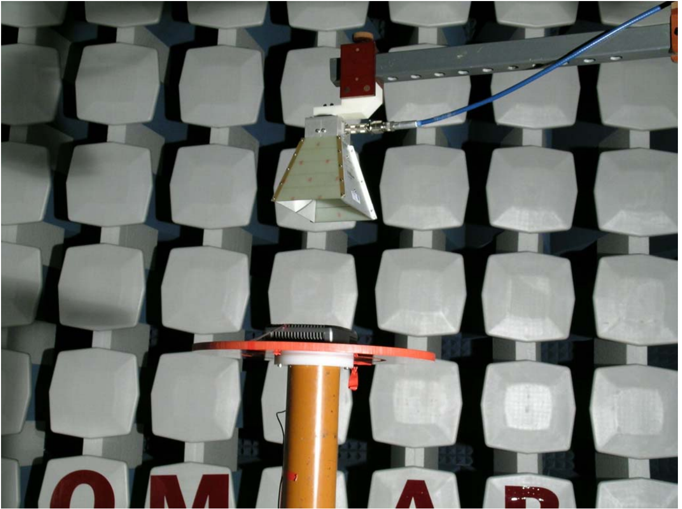
Fig 4 Test set-up when measuring electric field strength
