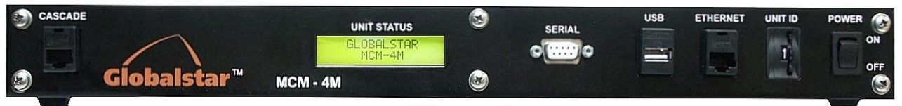
Figure 1-2 MCM-4M Multi Channel Modem – Front Panel
