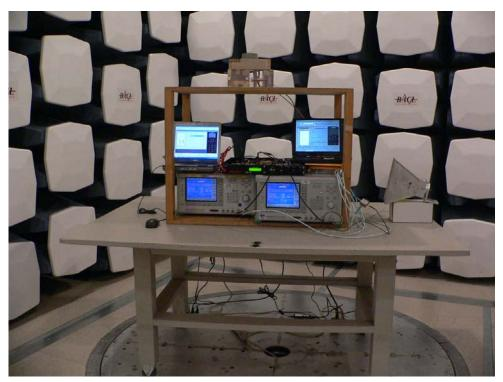
Transmitter Radiated Emission with 4. 5 dBi Antenna – Rear View
