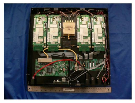
Modem Board with attached RF Board and shielding - Top View
