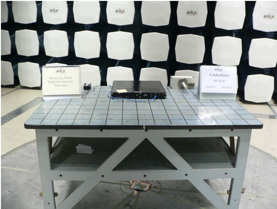
Radiated Setup – Receiver ( 10 m ) – Front View
