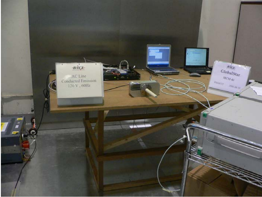
AC Lines Conducted Emission-Front View
