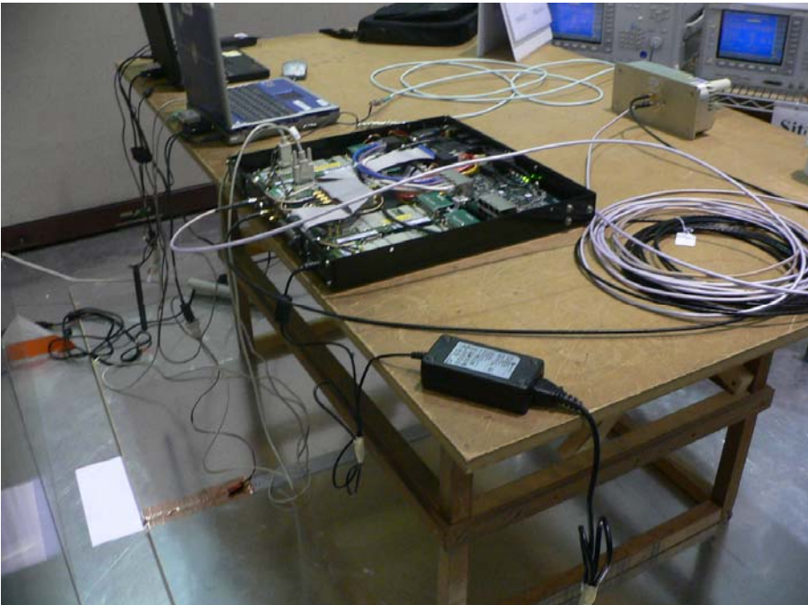
AC Lines Conducted Emission-Rear View
