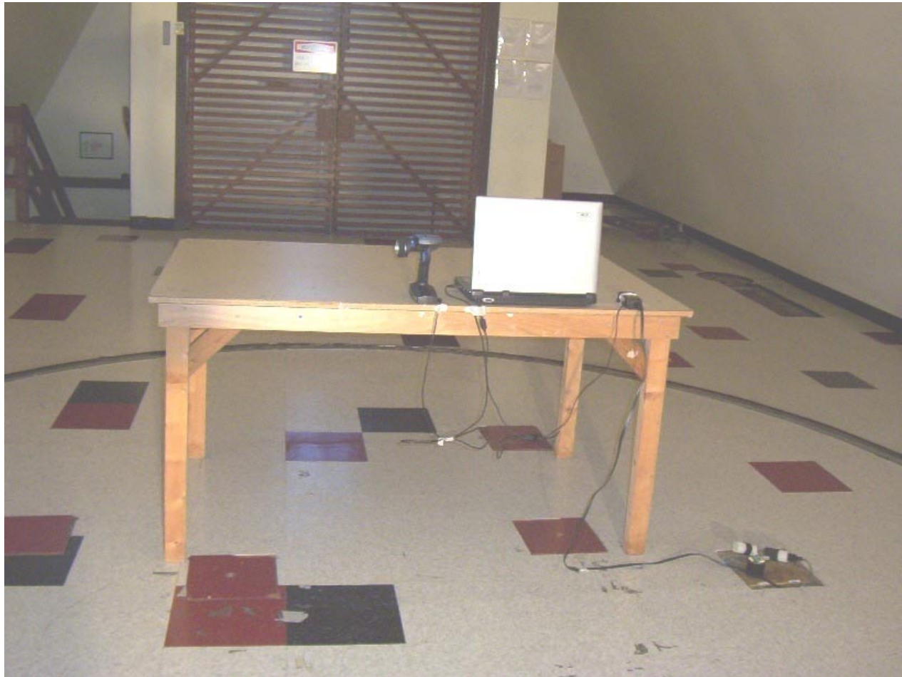
Photo 9: Radiated Emission Test Setup – EUT in USB Interface mode, Up Position View 1
