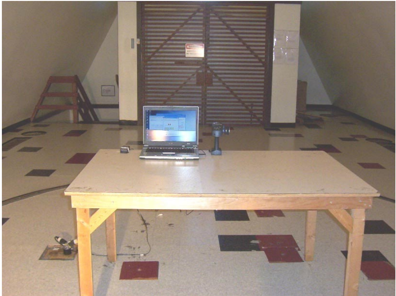
Photo 10: Radiated Emission Test Setup – EUT in USB Interface mode, Up Position View 2
