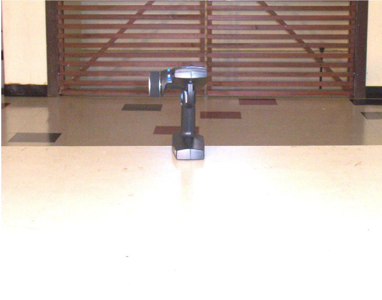
Photo 4: Radiated Emission Test Setup – EUT Standalone, Up Position View 2
