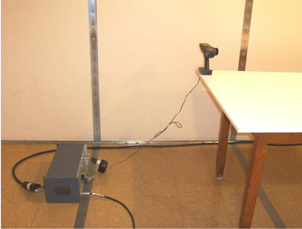
Photo 15: Conducted Emission Test Setup, Battery Charging Mode – Front View
