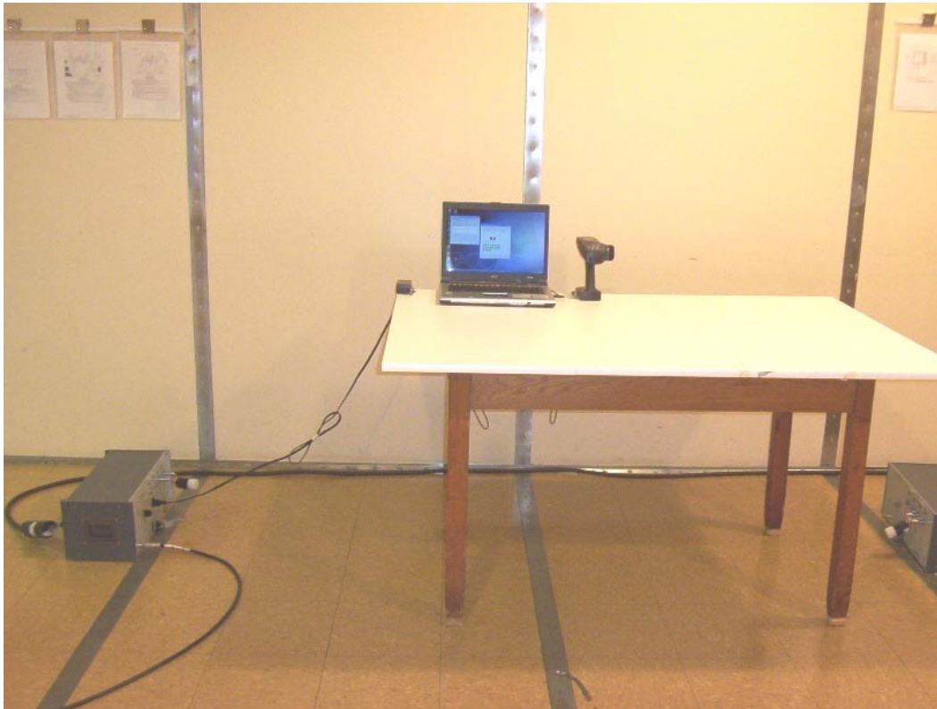
Photo 13: Conducted Emission Test Setup, USB Interface Mode – Front View
