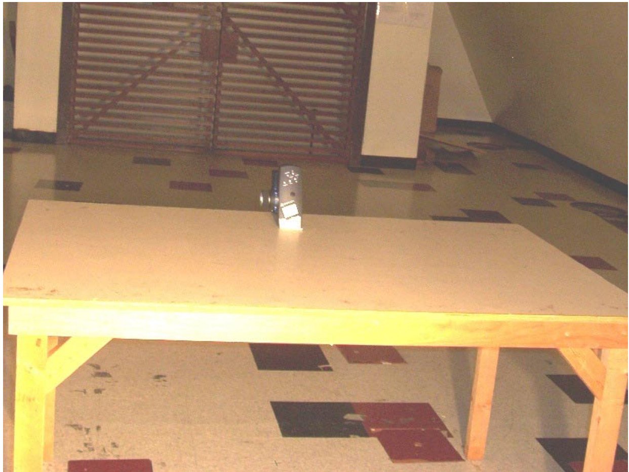
Photo 8: Radiated Emission Test Setup – EUT Standalone, Down Position View 2
