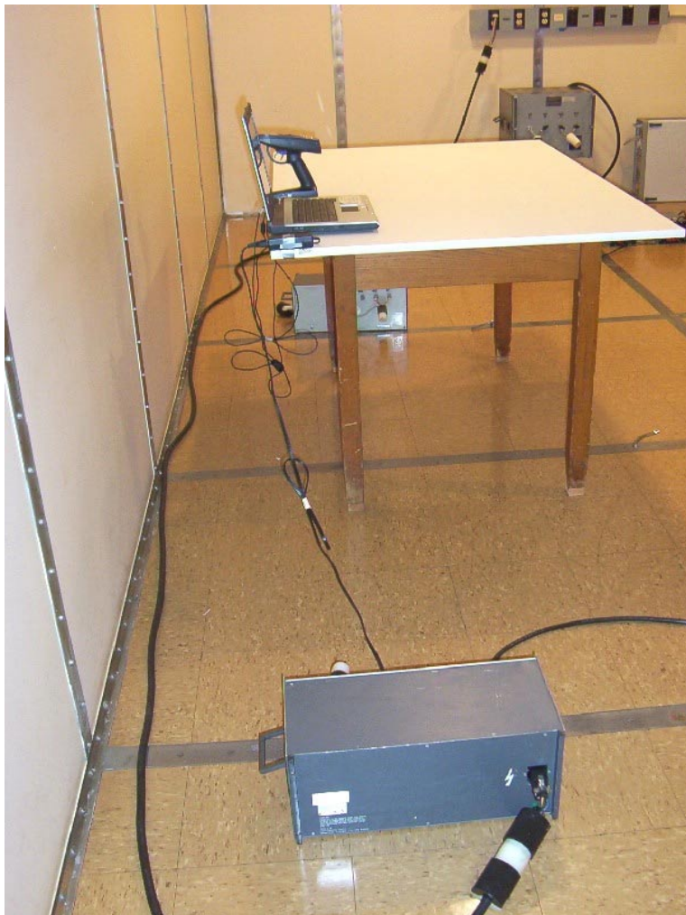
Photo 14: Conducted Emission Test Setup, USB Interface Mode – Side View
