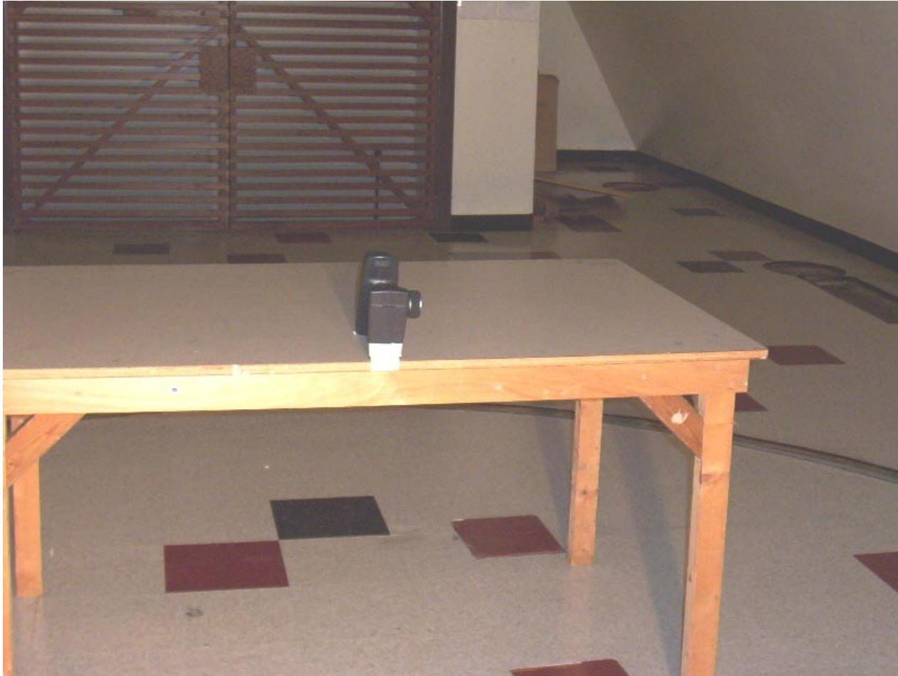
Photo 7: Radiated Emission Test Setup – EUT Standalone, Down Position View 1
