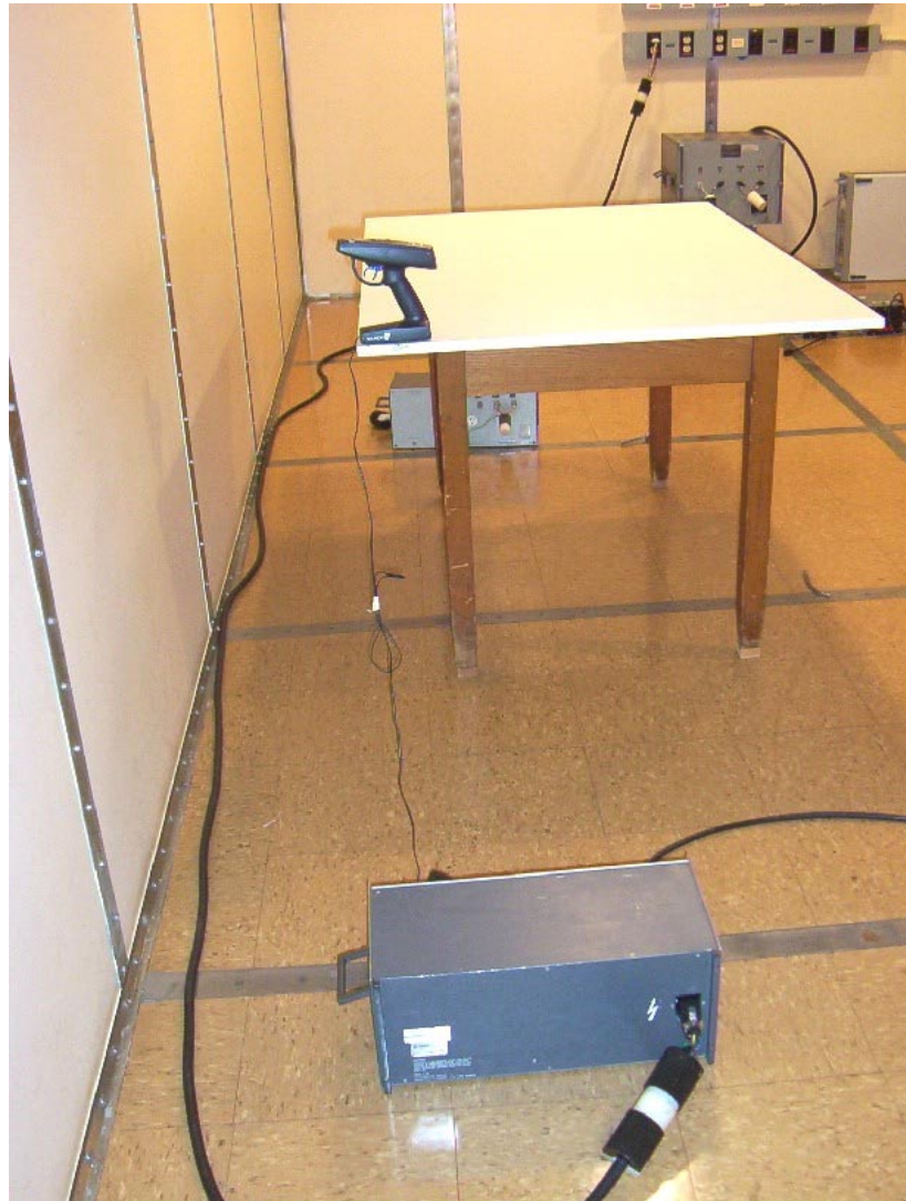
Photo 16: Conducted Emission Test Setup, Battery Charging Mode – Side View
