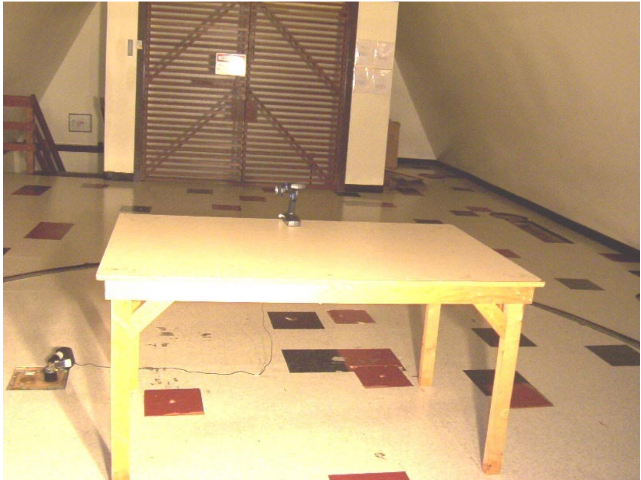
Photo 12: Radiated Emission Test Setup – EUT in Battery charging mode, Up Position View 2
