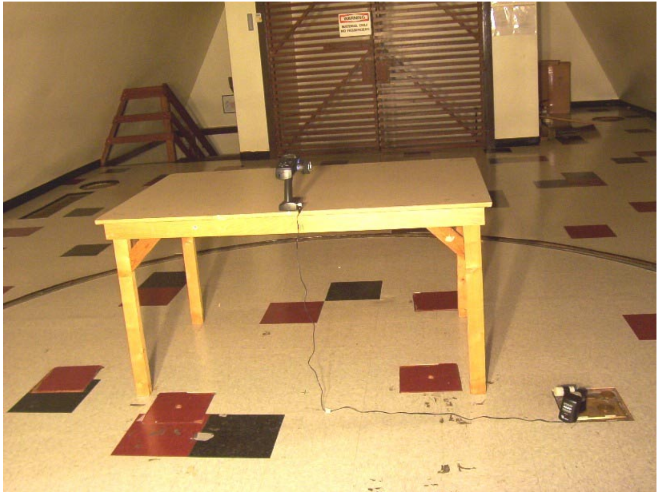
Photo 11: Radiated Emission Test Setup – EUT in Battery charging mode, Up Position View 1
