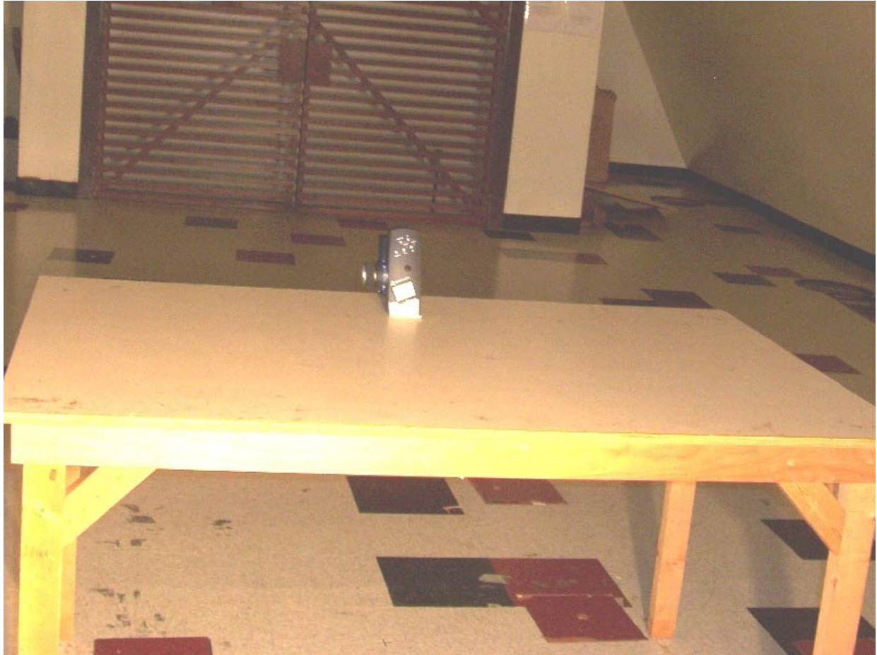
Photo 6: Radiated Emission Test Setup – EUT Standalone, Down Position View 2
