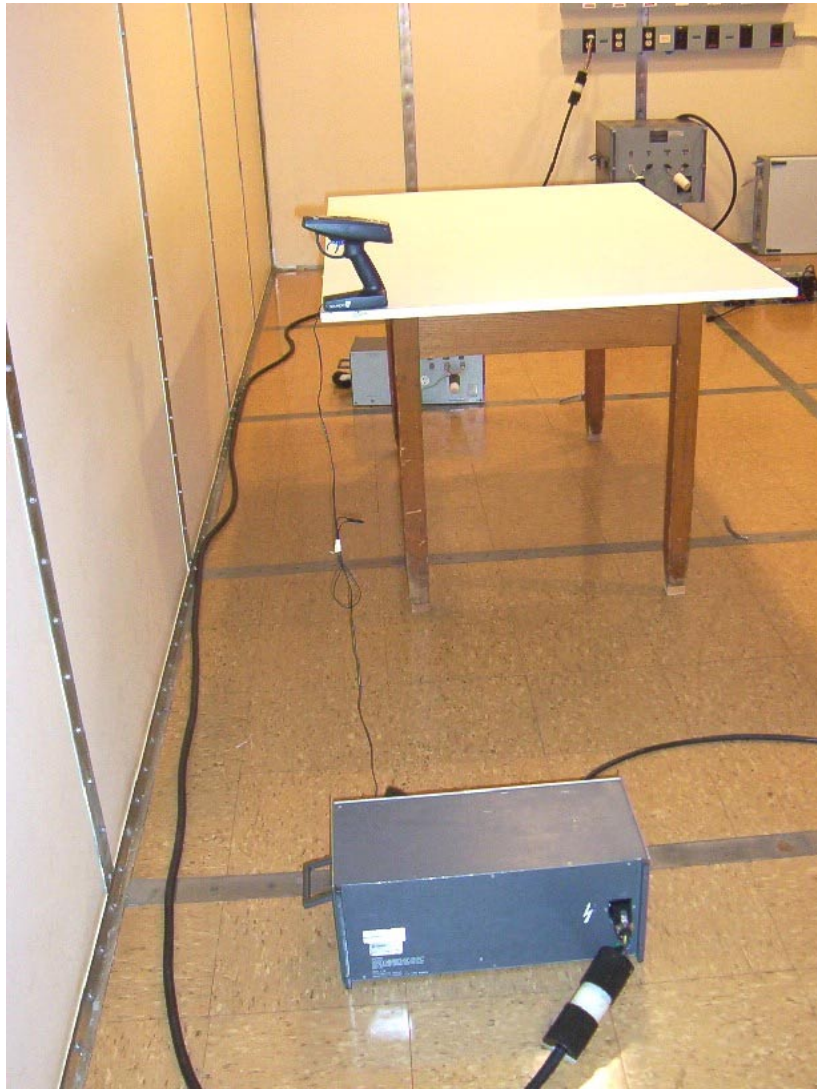
Photo 14: Conducted Emission Test Setup, Battery Charging Mode – Side View
