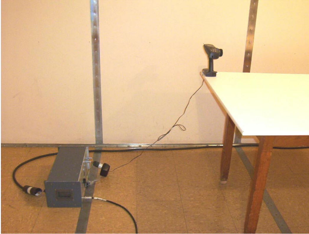
Photo 13: Conducted Emission Test Setup, Battery Charging Mode – Front View
