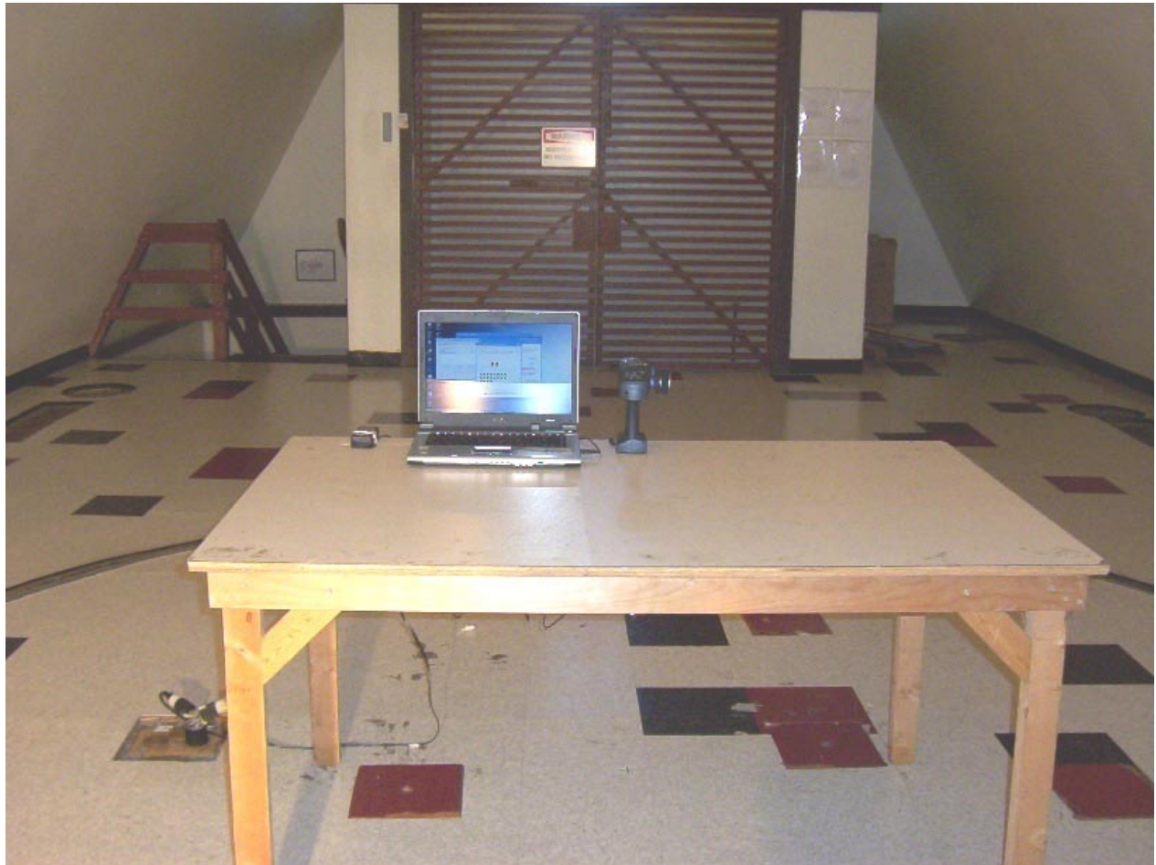
Photo 8: Radiated Emission Test Setup – EUT in USB Interface mode, Up Position View 2
