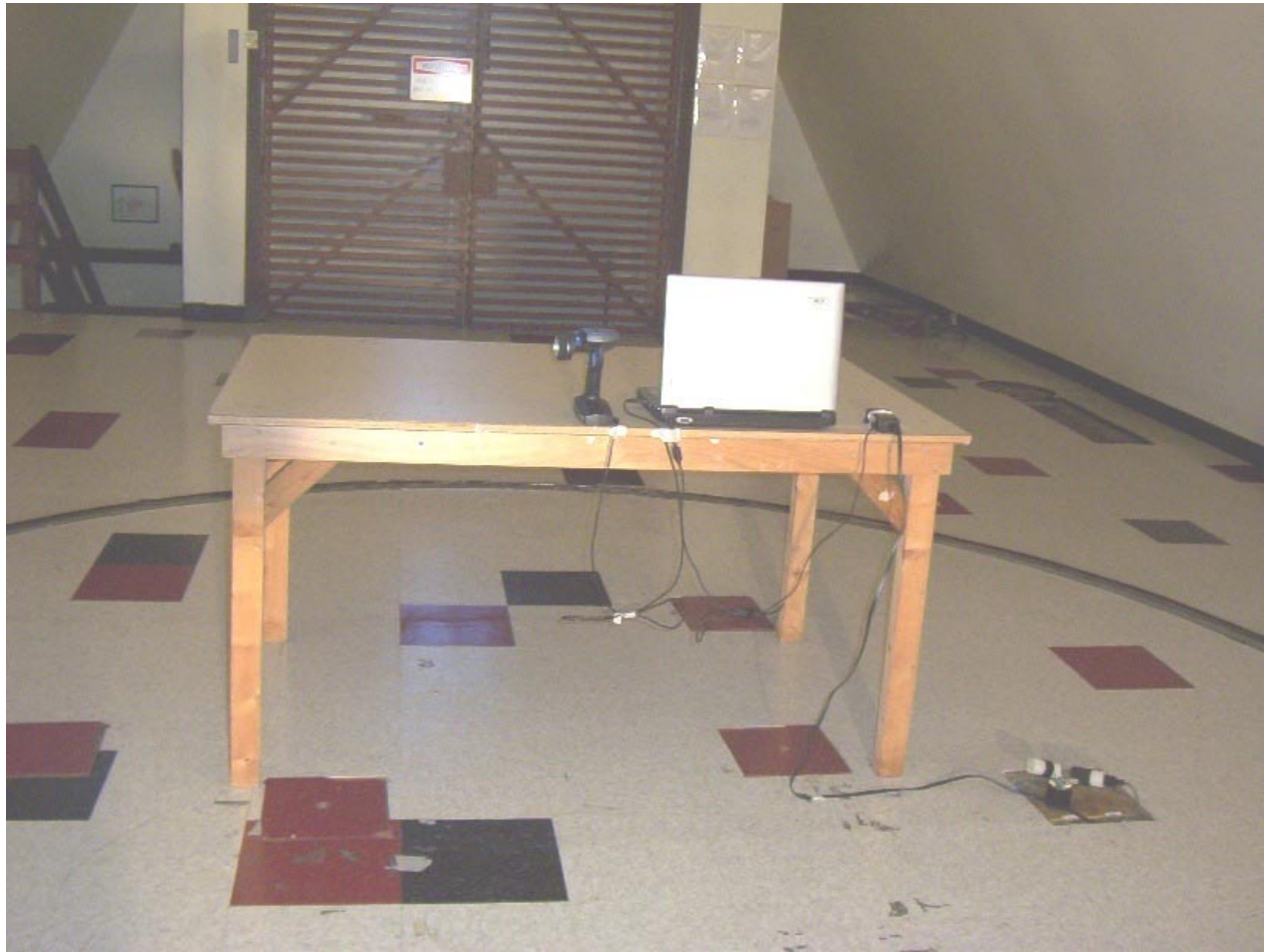
Photo 7: Radiated Emission Test Setup – EUT in USB Interface mode, Up Position View 1
