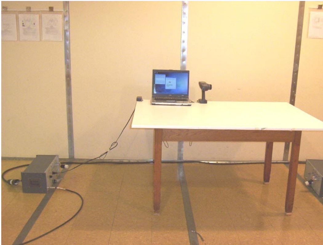
Photo 11: Conducted Emission Test Setup, USB Interface Mode – Front View
