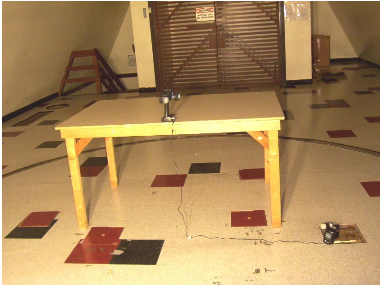
Photo 9: Radiated Emission Test Setup – EUT in Battery charging mode, Up Position View 1
