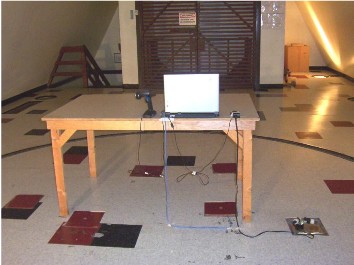
Photo 1: Radiated Emission Test Setup – USB Interface mode with Ethernet I/O at PC, Rear View
