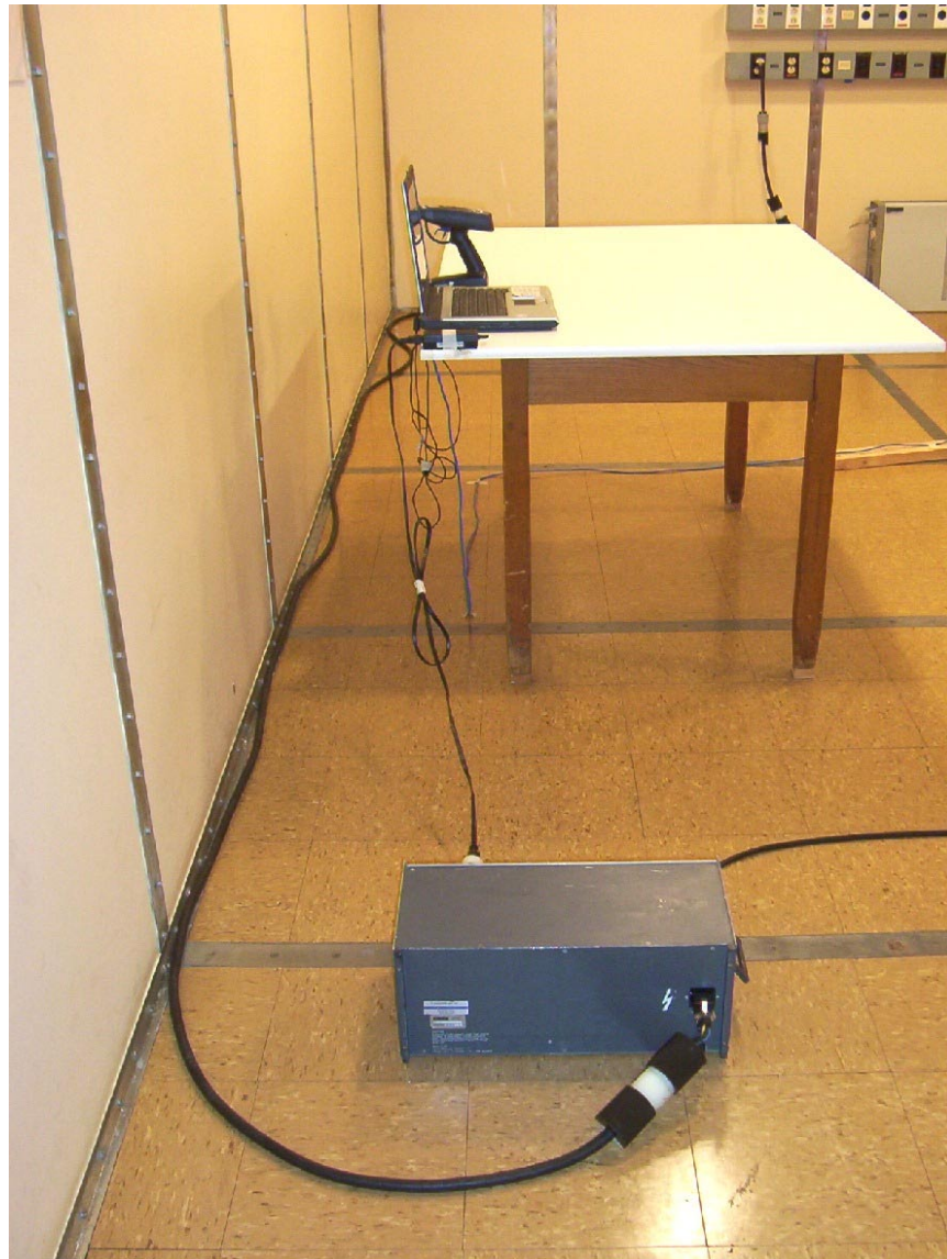
Photo 4: Conducted Emission Test Setup, USB Interface mode with Ethernet I/O at PC, Side View
