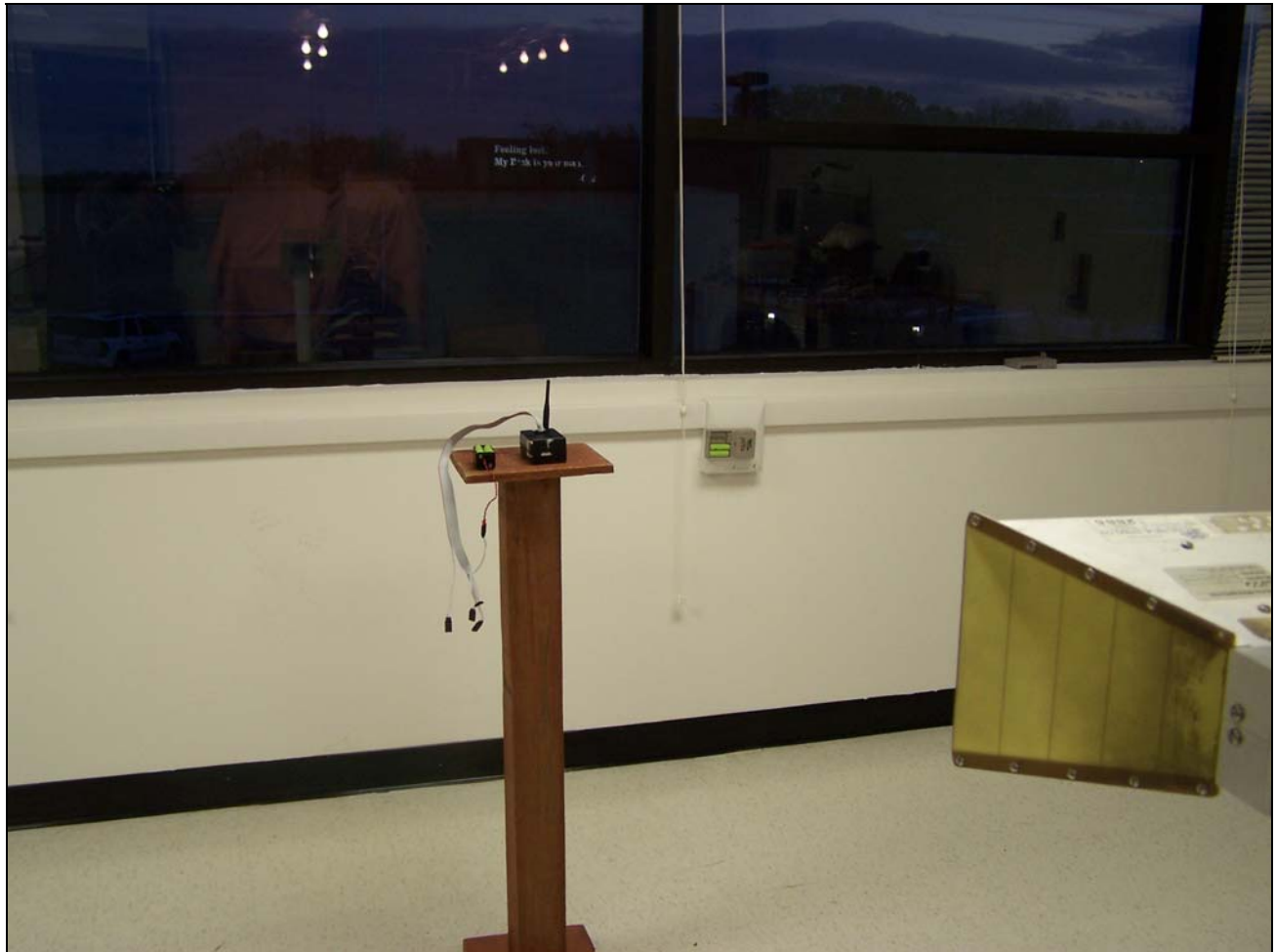
Photograph 2. Spurious Radiated Emissions 15.209, Test Setup
