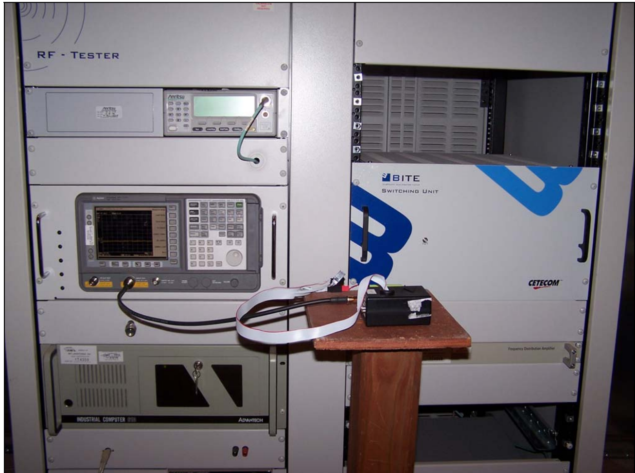
Photograph 4. Bandwidth and Channel Separation Test Setup
