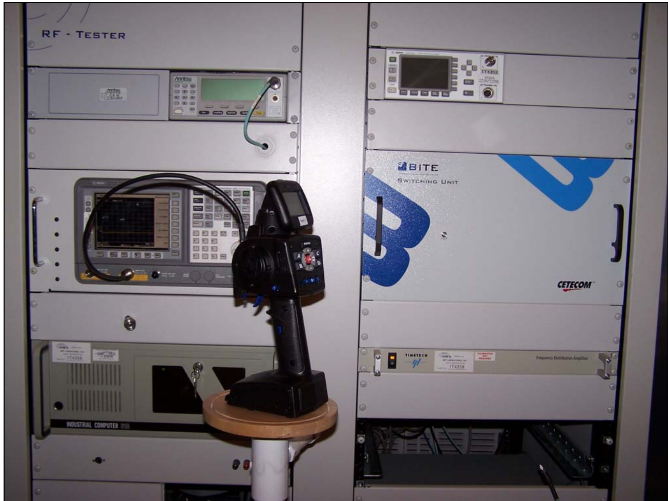
Photograph 4. Bandwidth and Channel Separation Test Setup
