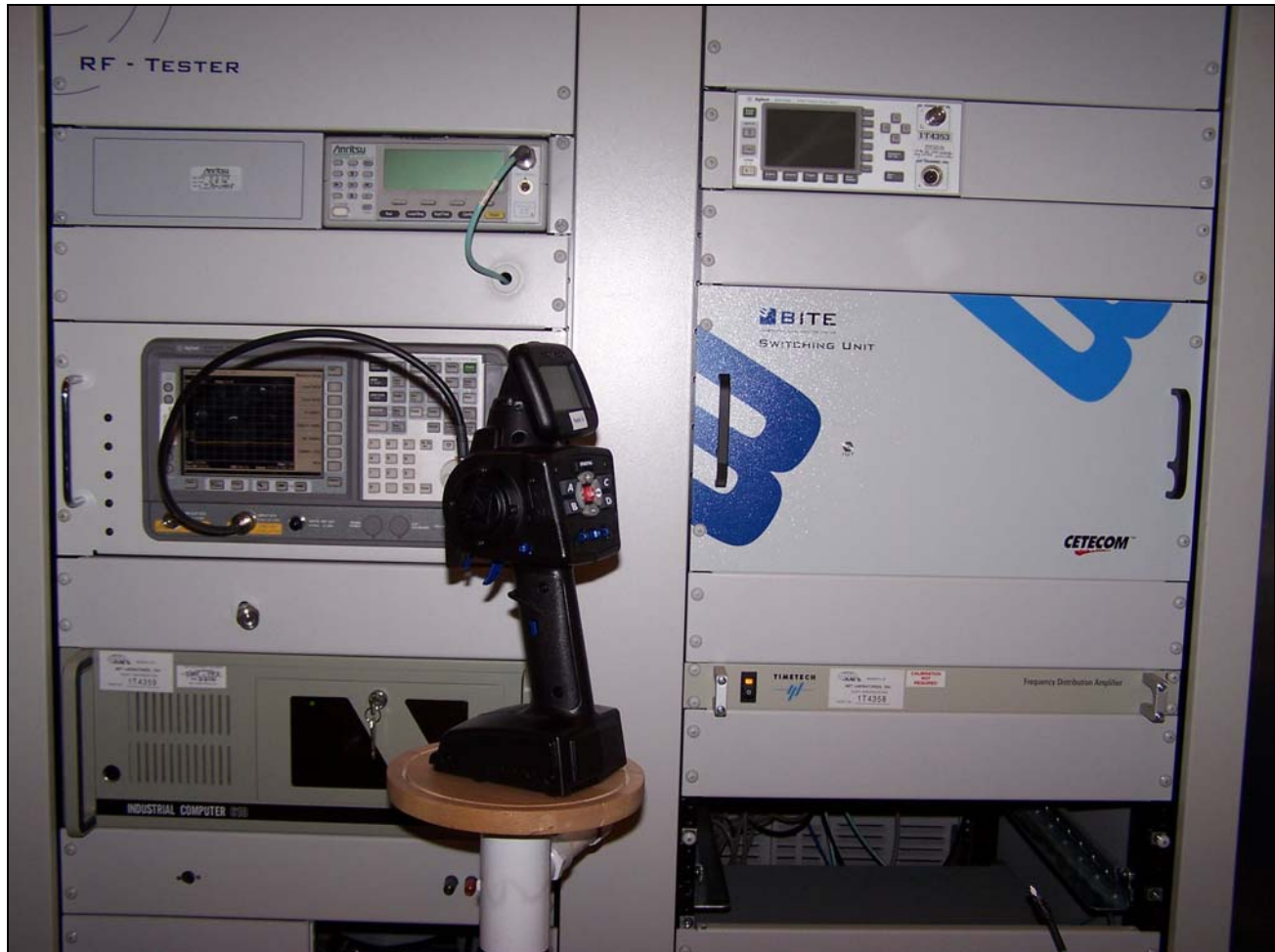
Photograph 5. Spurious Conducted Emissions Test setup
