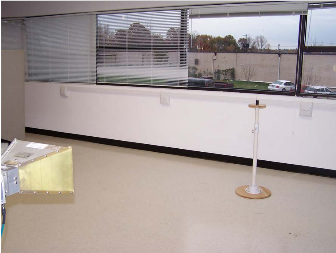
Photograph 6. Band Edge Measurements Test Setup
