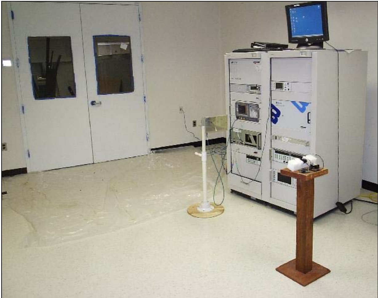
Photograph 3. Radiated Spurious Emission Test Setup
