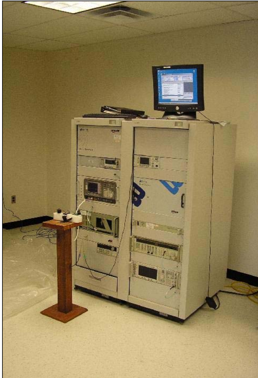
Photograph 5. Occupied Bandwidth Test Setup
