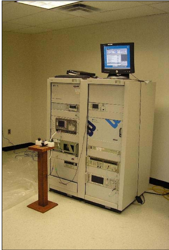
Photograph 7. Power Spectral Density Test setup
