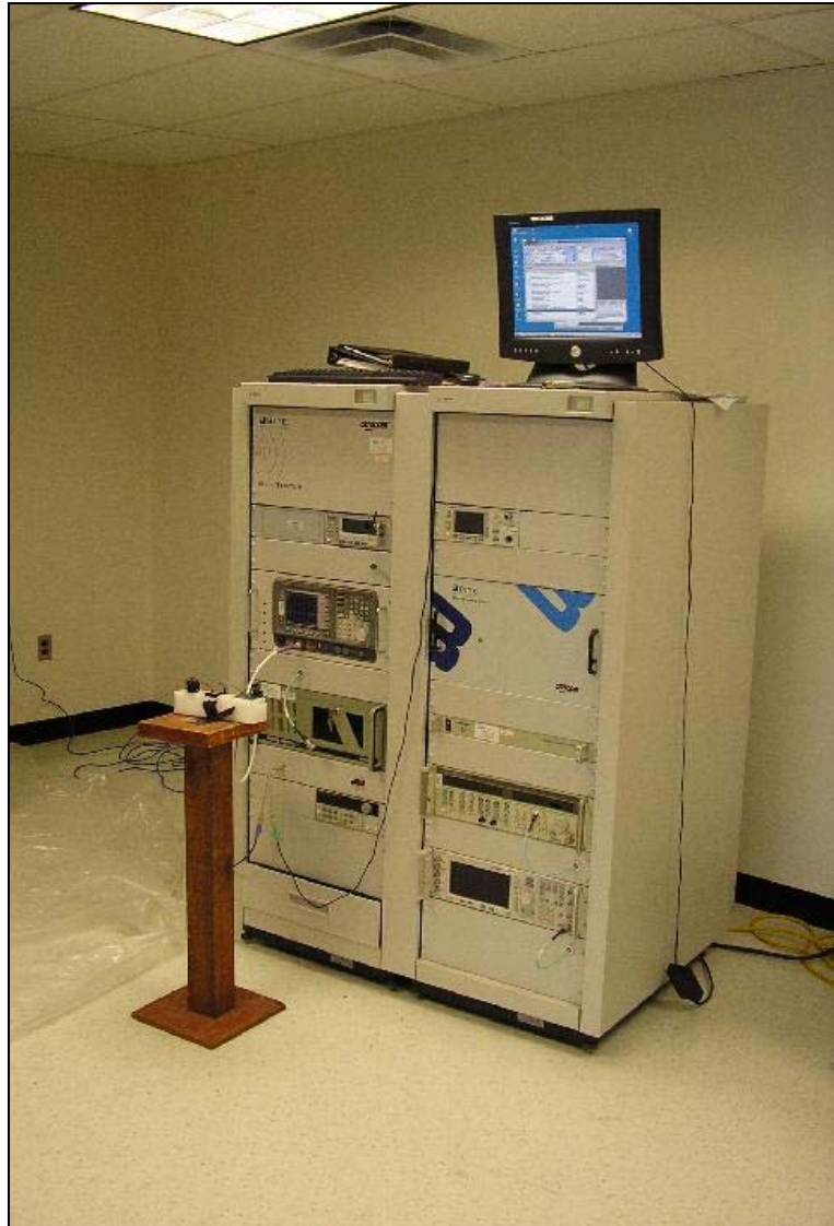
Photograph 8. Band Edge Measurements Test setup
