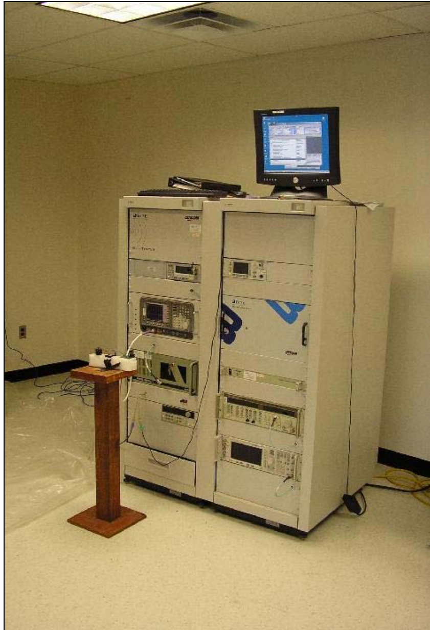
Photograph 6. Spurious Conducted Emissions Test setup
