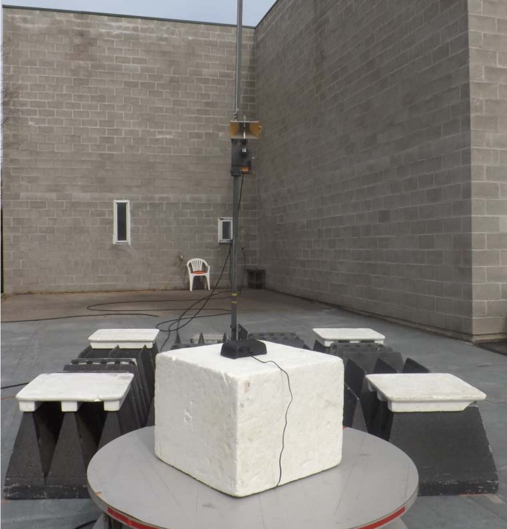
Figure E14.5 – Setup – Radiated Emissions 1 - 18GHz, Vertical
