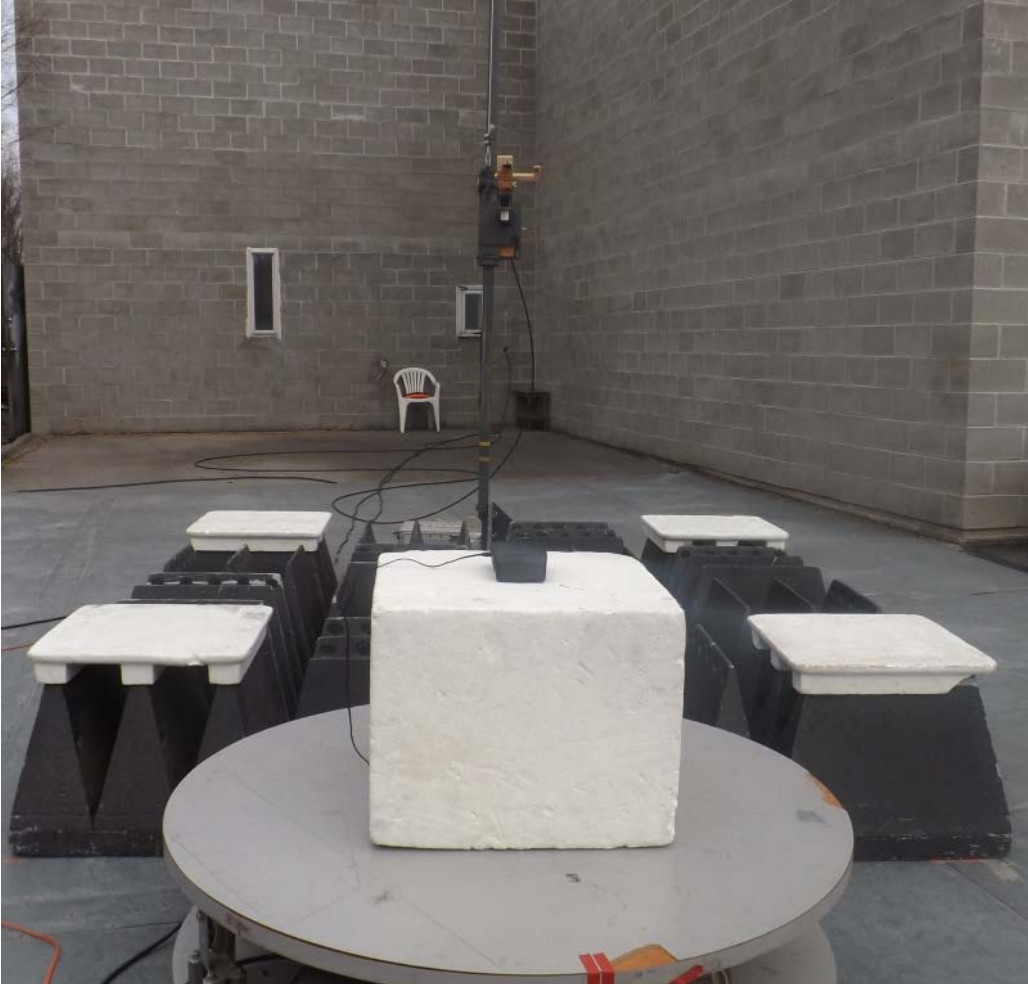
Figure E14.7 – Setup – Radiated Emissions 18 – 26.5GHz, Vertical
