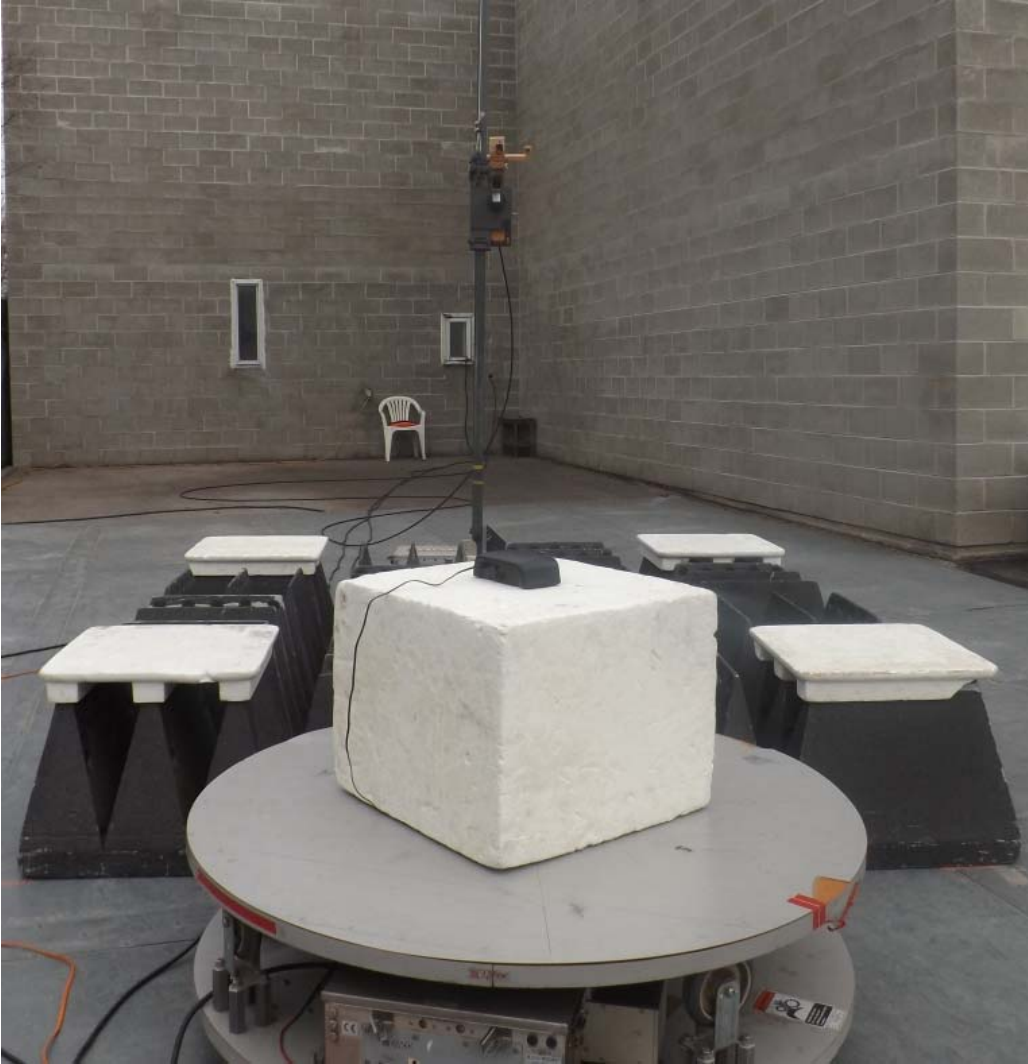
Figure E14.6 – Setup – Radiated Emissions 18 – 26.5GHz, Horizontal
