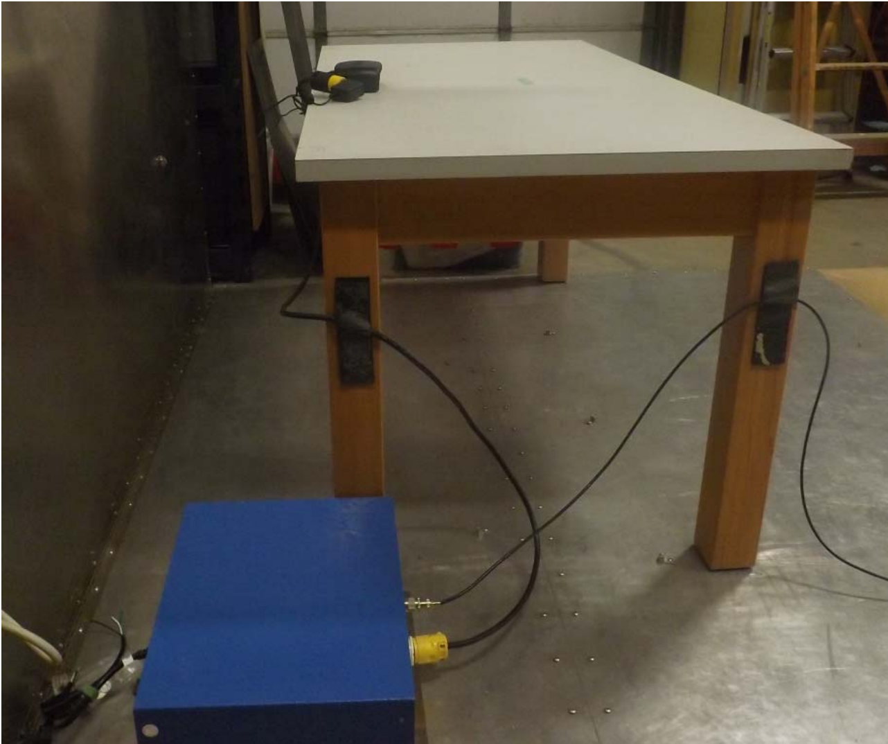
Figure E14.8 – Setup – Line Conducted Emissions
