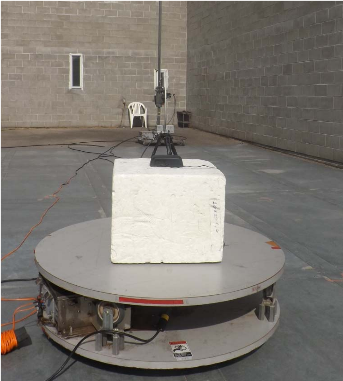
Figure E14.2 – Setup – Radiated Emissions < 30MHz, Side
