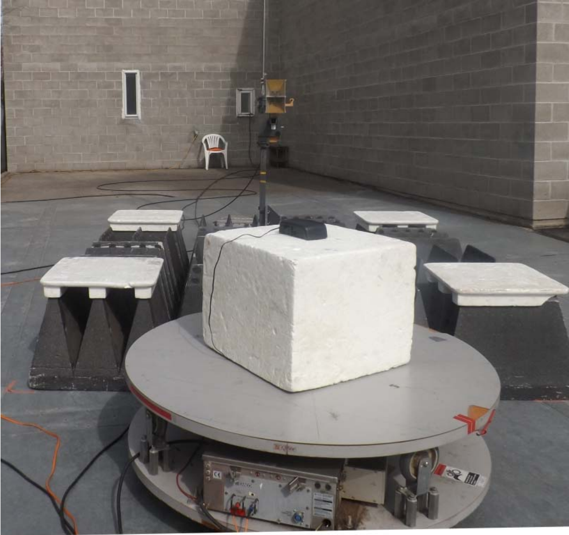
Figure E14.4 – Setup – Radiated Emissions 1 - 18GHz, Horizontal
