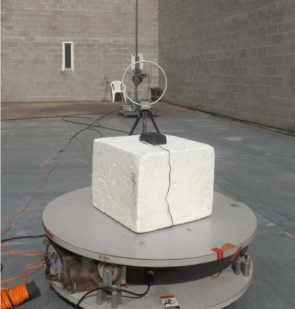
Figure E14.1 – Setup – Radiated Emissions < 30MHz, Front
