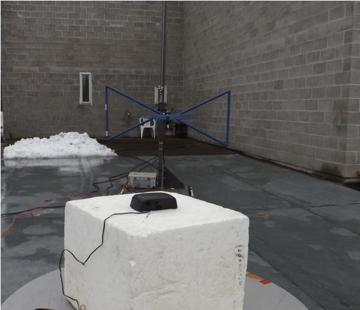
Figure E14.3 – Setup – Radiated Emissions < 1GHzHz, Horizontal
