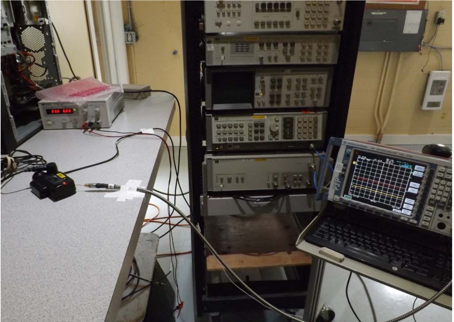
Figure E23.1 – Setup Photo – Conducted Measurements
