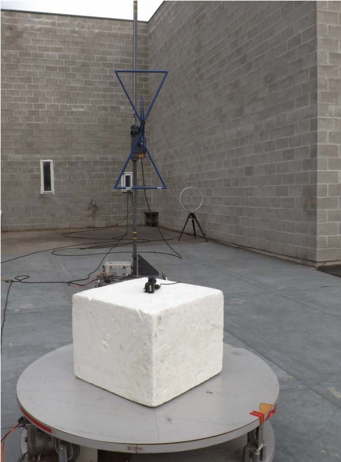
Figure E23.3 – Setup Photo – Radiated Measurements, 30 – 1000MHz
