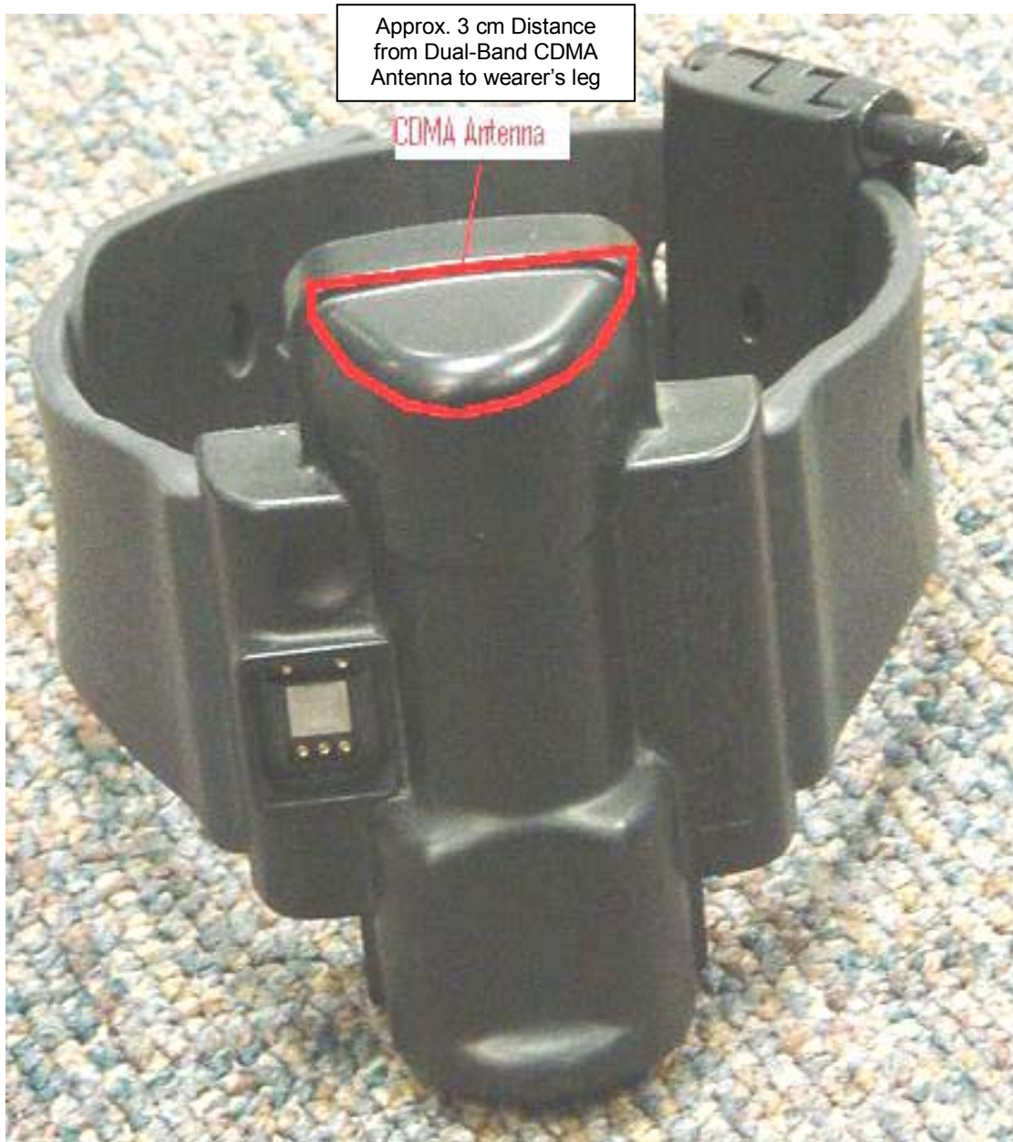
Ankle-worn Offender Tracking Bracelet with GPS Receiver & Dual-Band CDMA Transceiver
