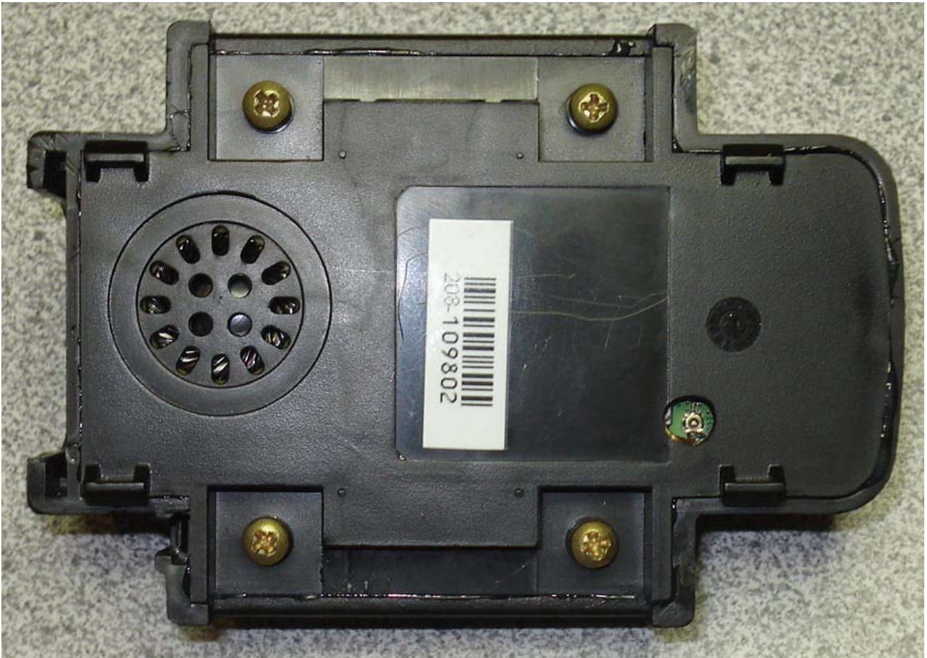
Ankle-worn Offender Tracking Bracelet with ankle-strap and back plate removed (showing 4 metal screws)
